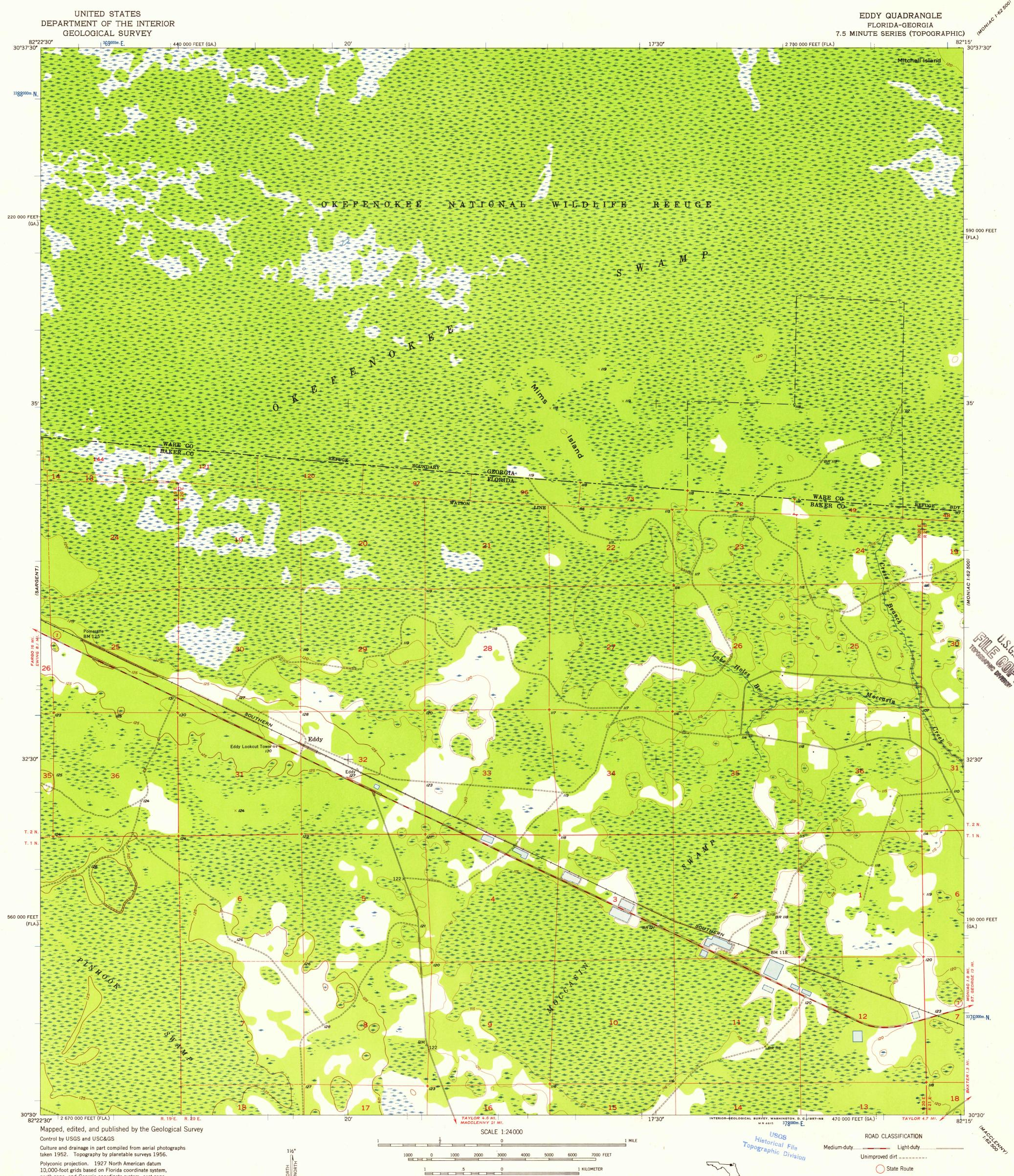
10,000-foot grids based on Florida coordinate system, north zone, and Georgia coordinate system, east zone 1000 meter Universal Transverse Mercator Grid ticks, Zone 17, shown in blue
