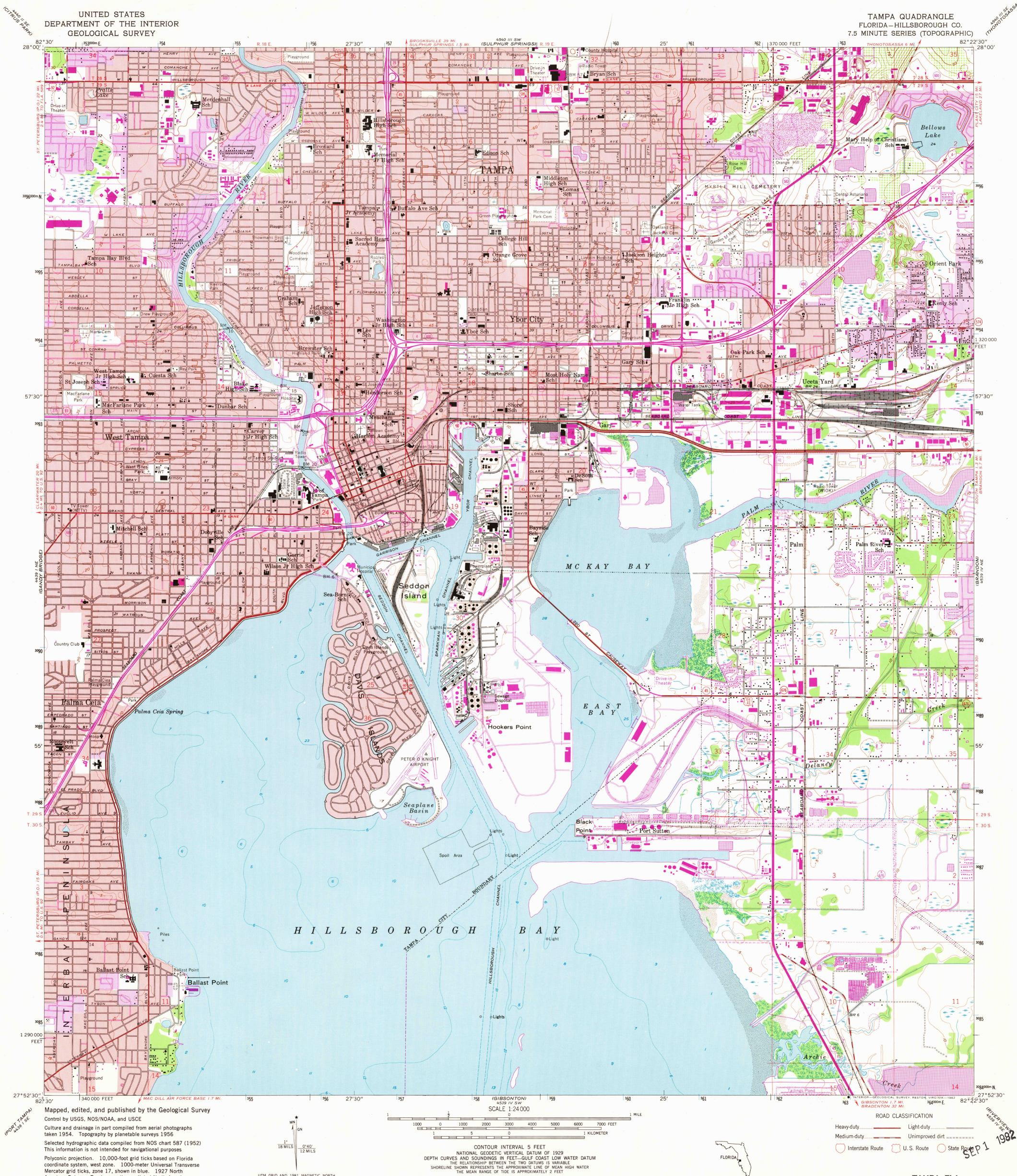
Polyconic projection. 10,000-foot grid ticks based on Florida coordinate system, west zone. 1000-meter Universal Transverse Mercator grid ticks, zone 17, shown in blue. 1927 North American Datum. To place on the predicted North American Datum 1983 move the projection lines 29 meters south and 17 meters west as shown by dashed corner ticks
