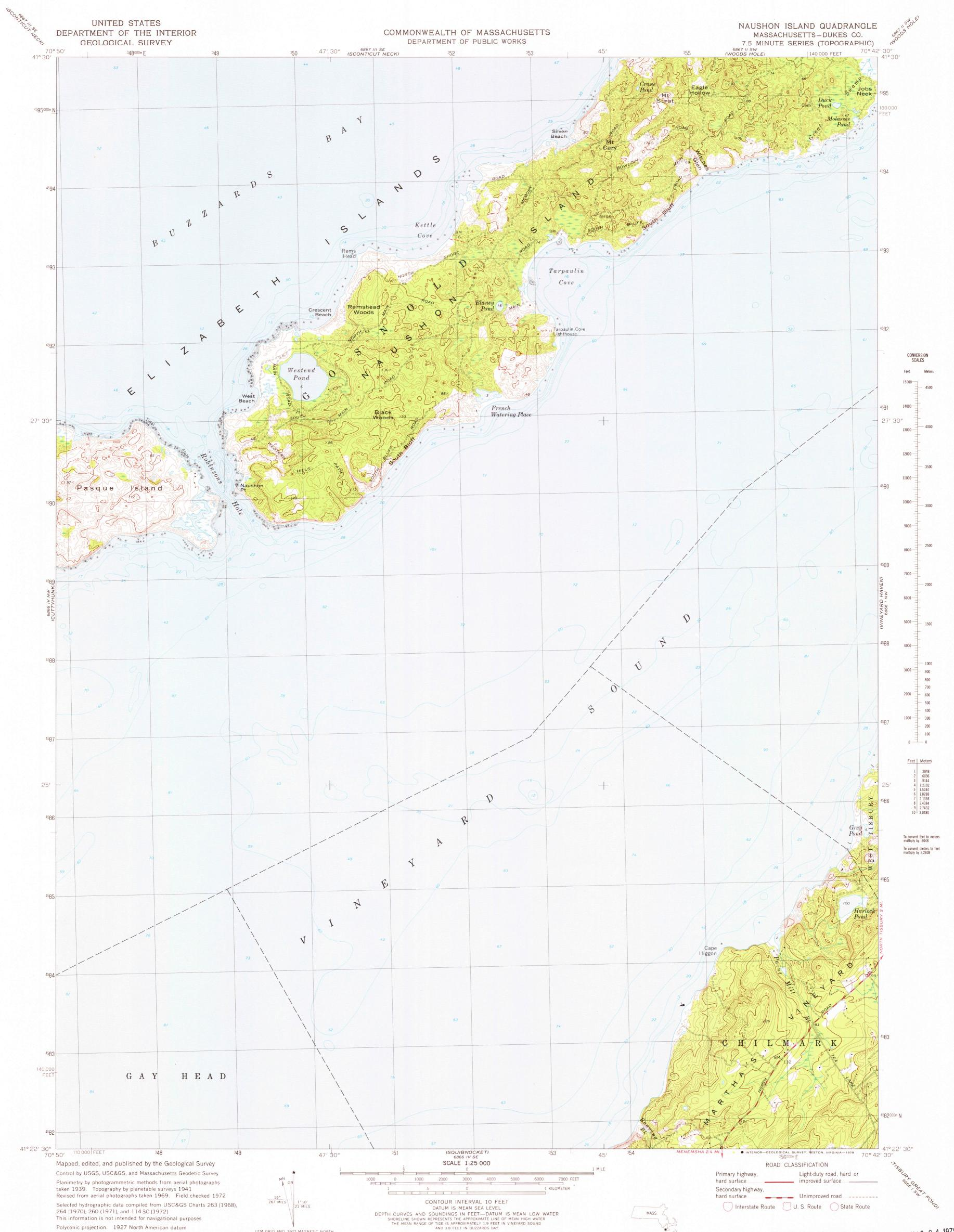
Polyconic projection. 1927 North American datum UTM GRID AND 1972 MAGNETIC NORTH DECLINATION AT CENTER OF SHEET 10,000-foot grid based on Massachusetts coordinate system, island zone 1000-meter Universal Transverse Mercator grid, zone 19
