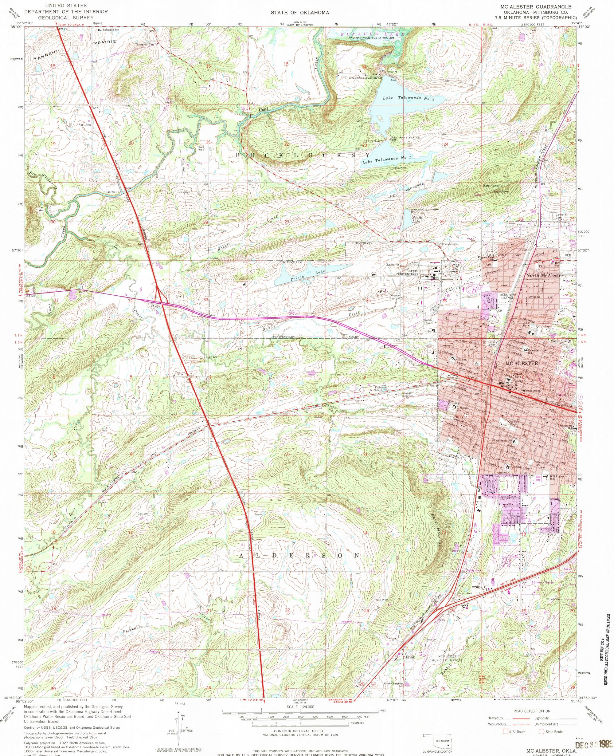
zone 15, shown in blue To place on the predicted North American Datum 1983 move the projection lines 6 meters south and 23 meters east as shown by dashed corner ticks
