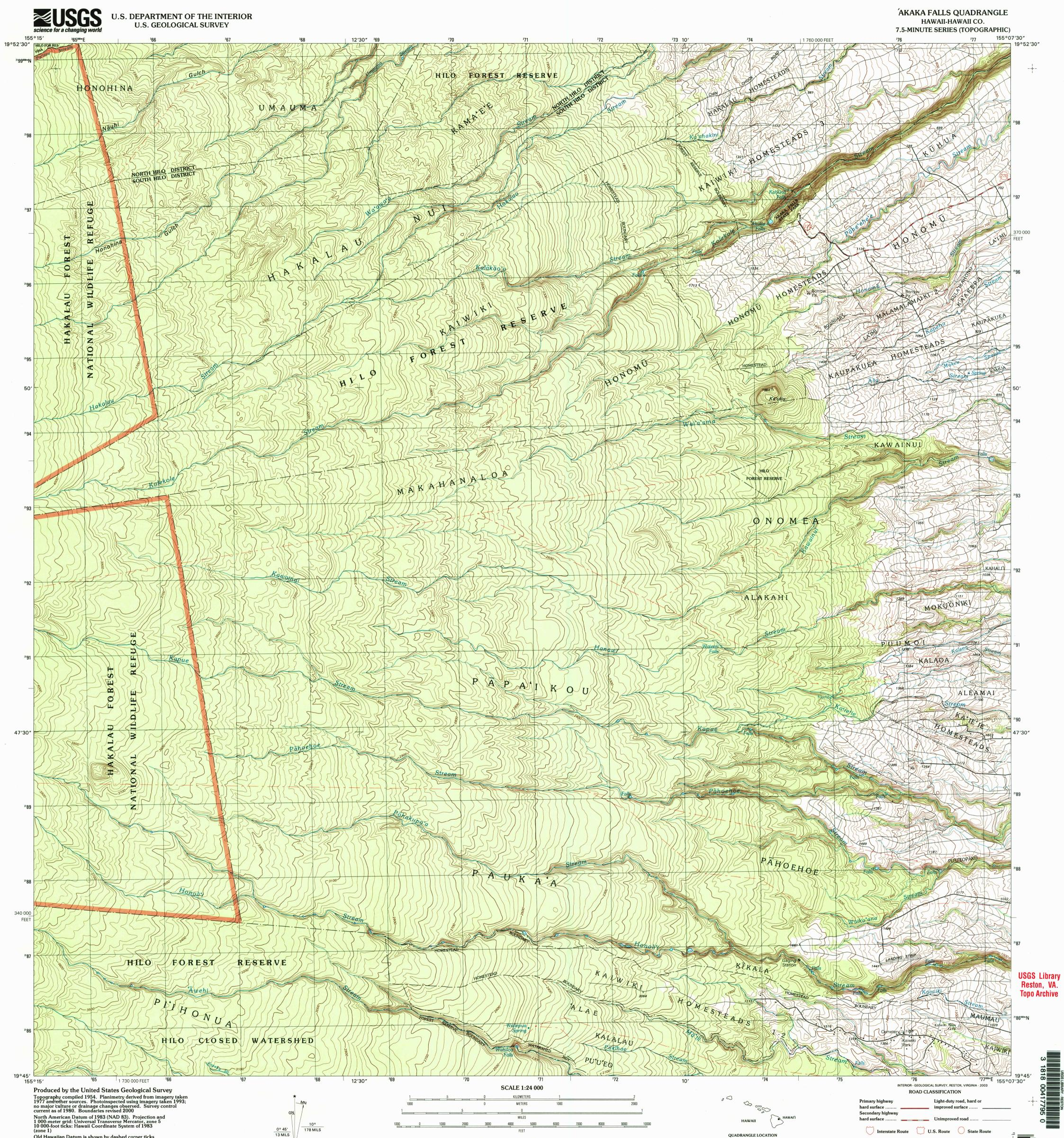
Old Hawaiian Datum is shown by dashed corner ticks The values of the shift between NAD 83 and Old Hawaiian Datum for 7.5-minute intersections are obtainable from National Geodetic Survey NADCON software
