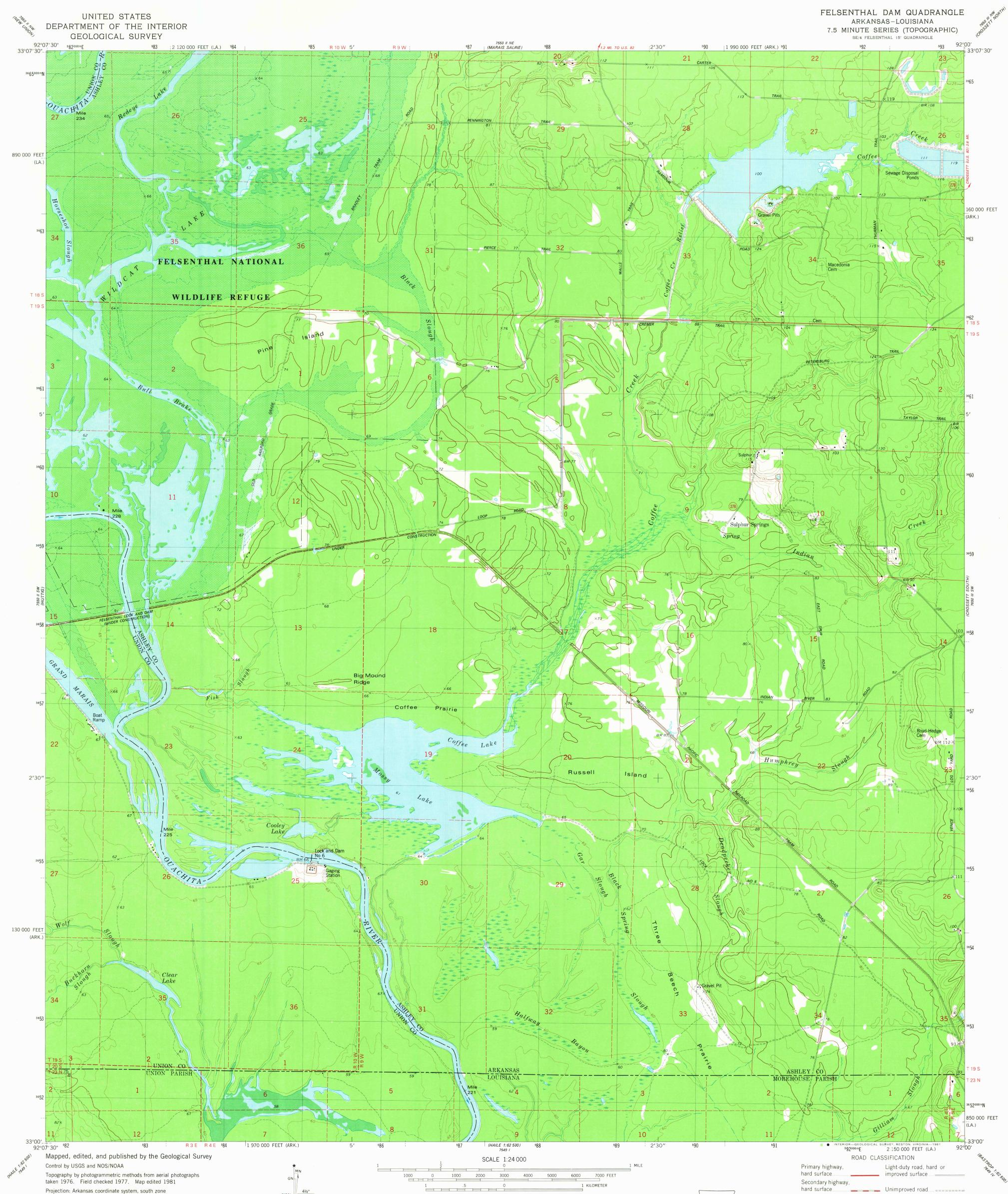
(Lambert conformal conic) 10,000-foot grid ticks based on Arkansas coordinate system, south zone and Louisiana coordinate system, north zone 1000-meter Universal Transverse Mercator grid, zone 15 1927 North American Datum To place on the predicted North American Datum 1983 move the projection lines 11 meters south and 13 meters east as shown by dashed corner ticks There may be private inholdings within the boundaries of the National or State reservations shown on this map
