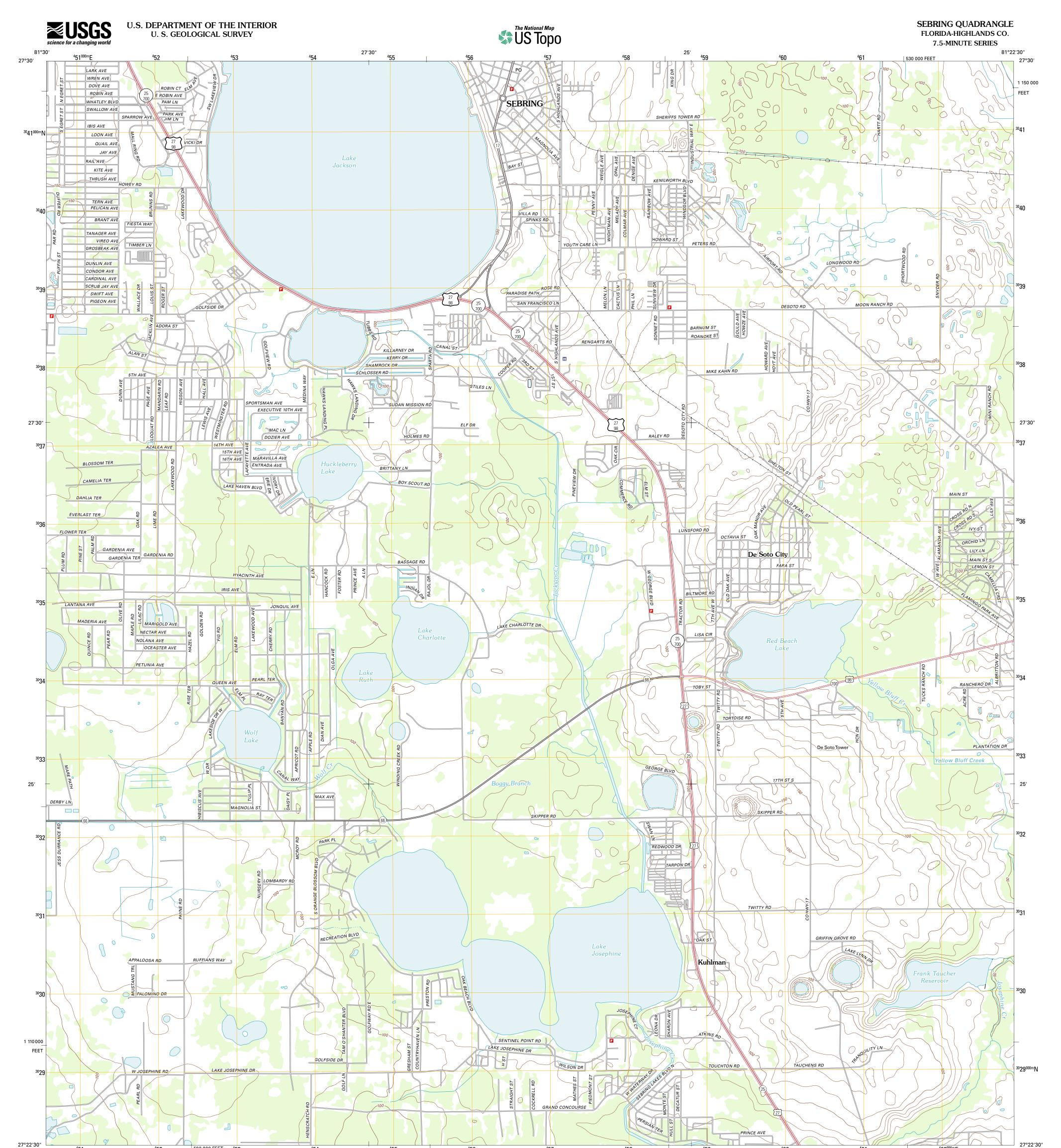
Produced by the United States Geological Survey North American Datum of 1983 (NAD83) World Geodetic System of 1984 (WGS84). Projection and 1 000-meter grid: Universal Transverse Mercator, Zone 17R 10 000-foot ticks: Florida Coordinate System of 1983 (east zone)
