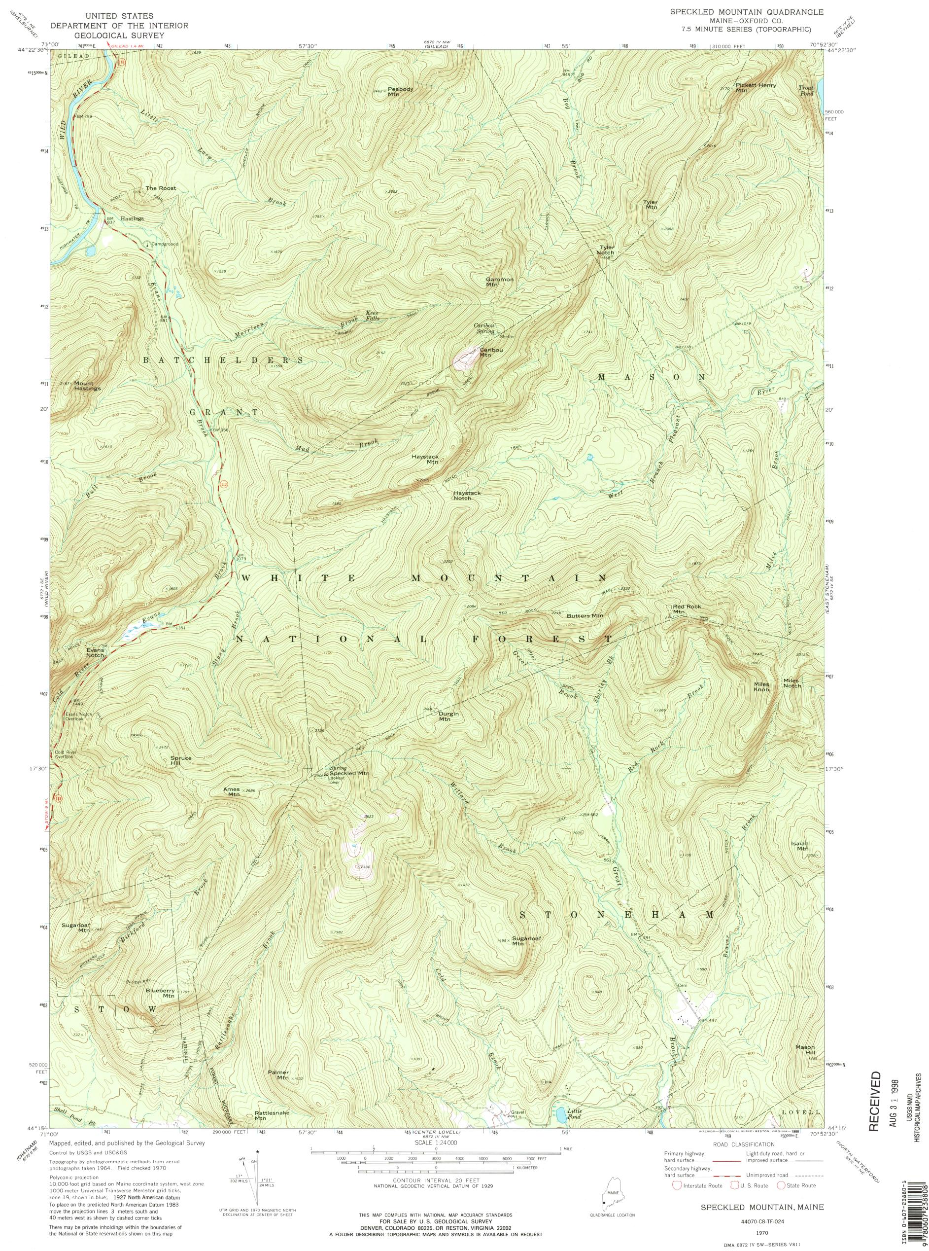
10,000-foot grid based on Maine coordinate system, west zone 1000-meter Universal Transverse Mercator grid ticks, zone 19, shown in blue. 1927 North American datum To place on the predicted North American Datum 1983 move the projection lines 3 meters south and 40 meters west as shown by dashed corner ticks
