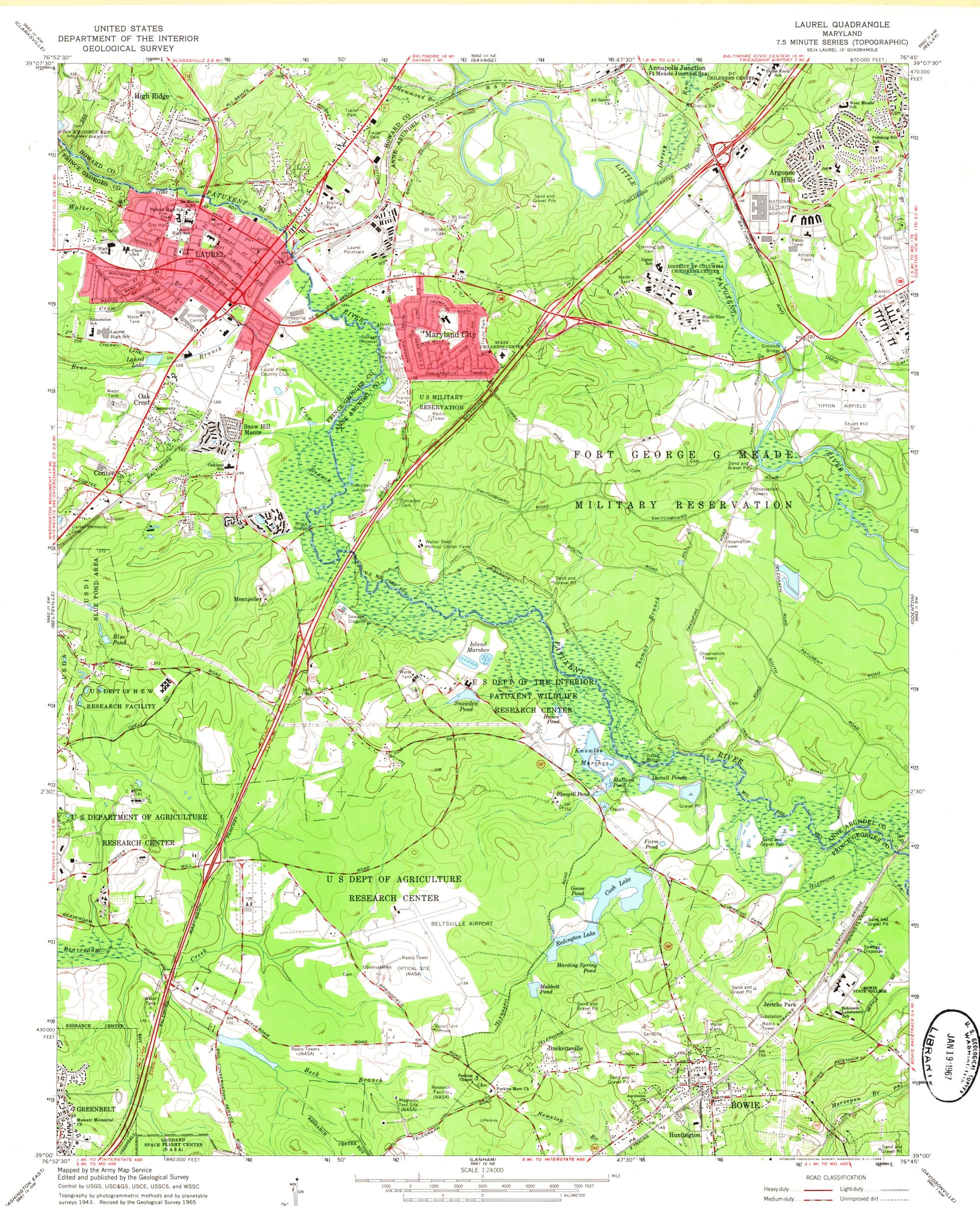
Topography by photogrammetric methods and by planetable surveys 1943. Revised by the Geological Survey 1965 Polyconic projection. 1927 North American datum 10,000-foot grid based on Maryland coordinate system 1000-meter Universal Transverse Mercator grid ticks, zone 18, shown in blue
