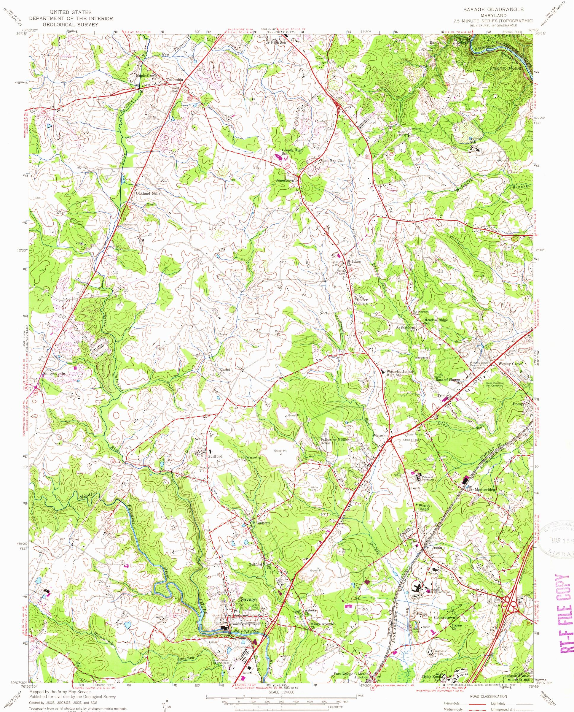
Topography from aerial photographs by photogrammetric methods and by planetable surveys 1943. Planimetric detail revised from aerial photographs taken 1955. Field check 1957
