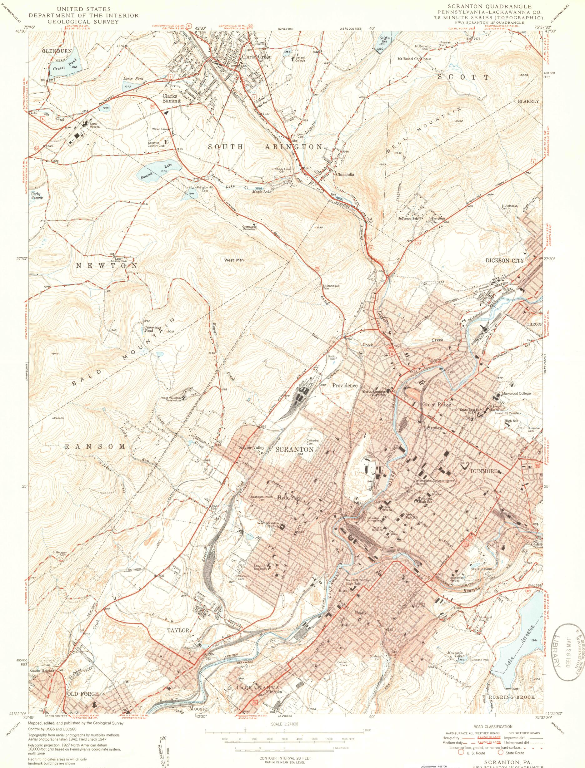
Polyconic projection. 1927 North American datum 10,000-foot grid based on Pennsylvania coordinate system, north zone Red tint indicates areas in which only landmark buildings are shown Contours in strip mine areas compiled from 1942 photography
