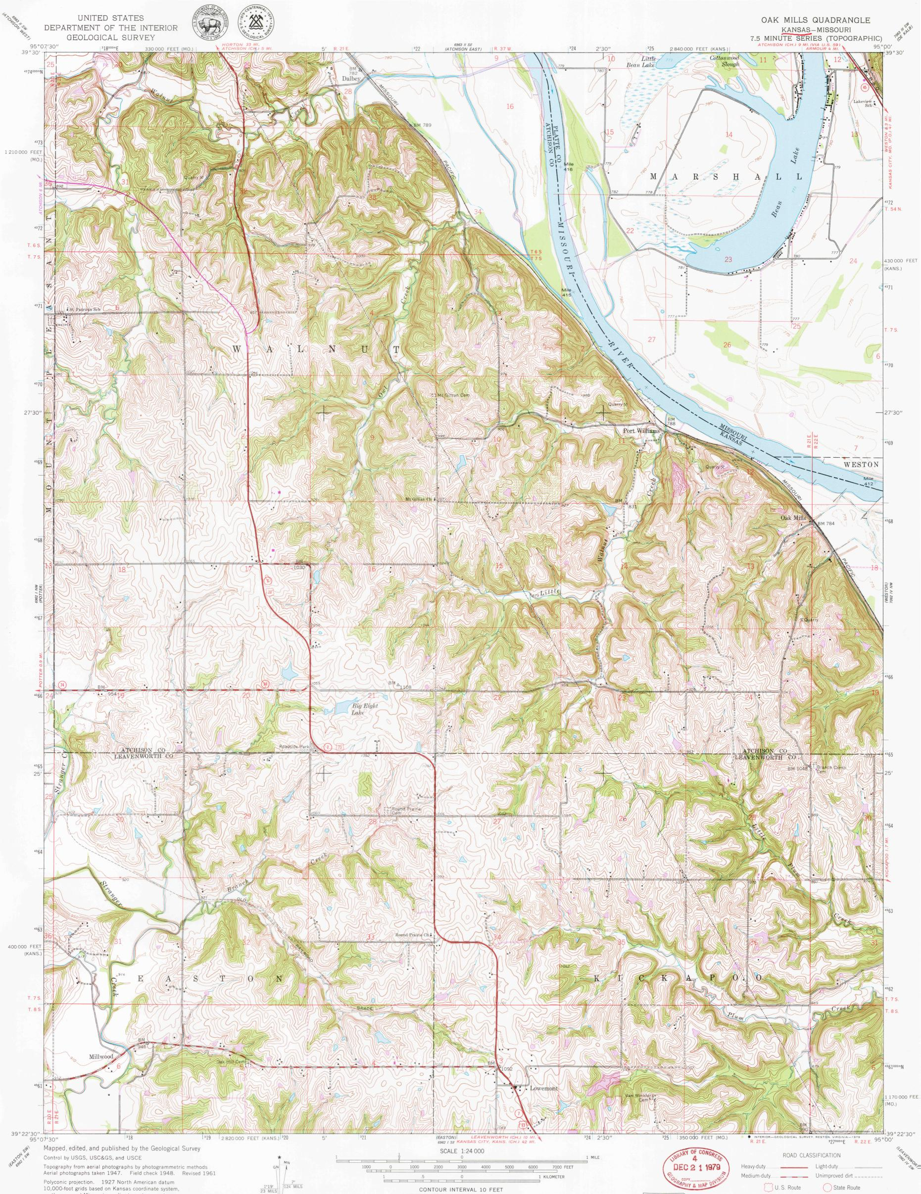
10,000-foot grids based on Kansas coordinate system, north zone, and Missouri coordinate system, west zone To place on the predicted North American Datum 1983 move the projection lines 4 meters north and 21 meters east as shown by dashed corner ticks 1000-meter Universal Transverse Mercator grid ticks, zone 15, shown in blue
