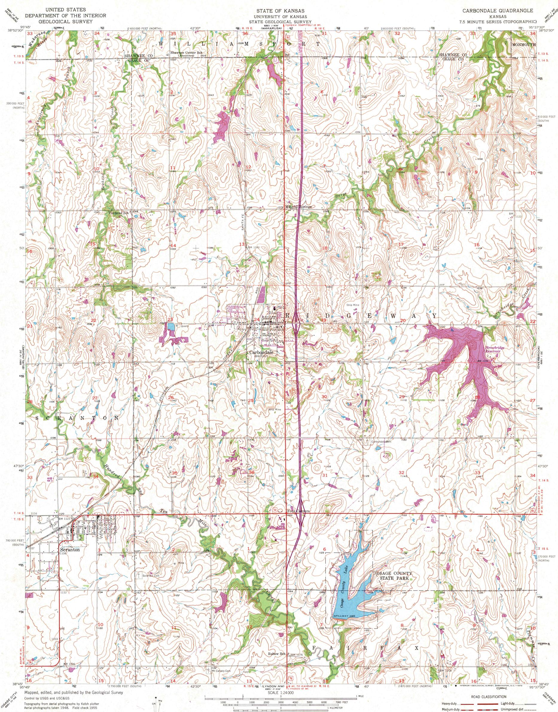
Polyconic projection. 1927 North American datum 10,000-foot grids based on Kansas coordinate system, north and south zones
