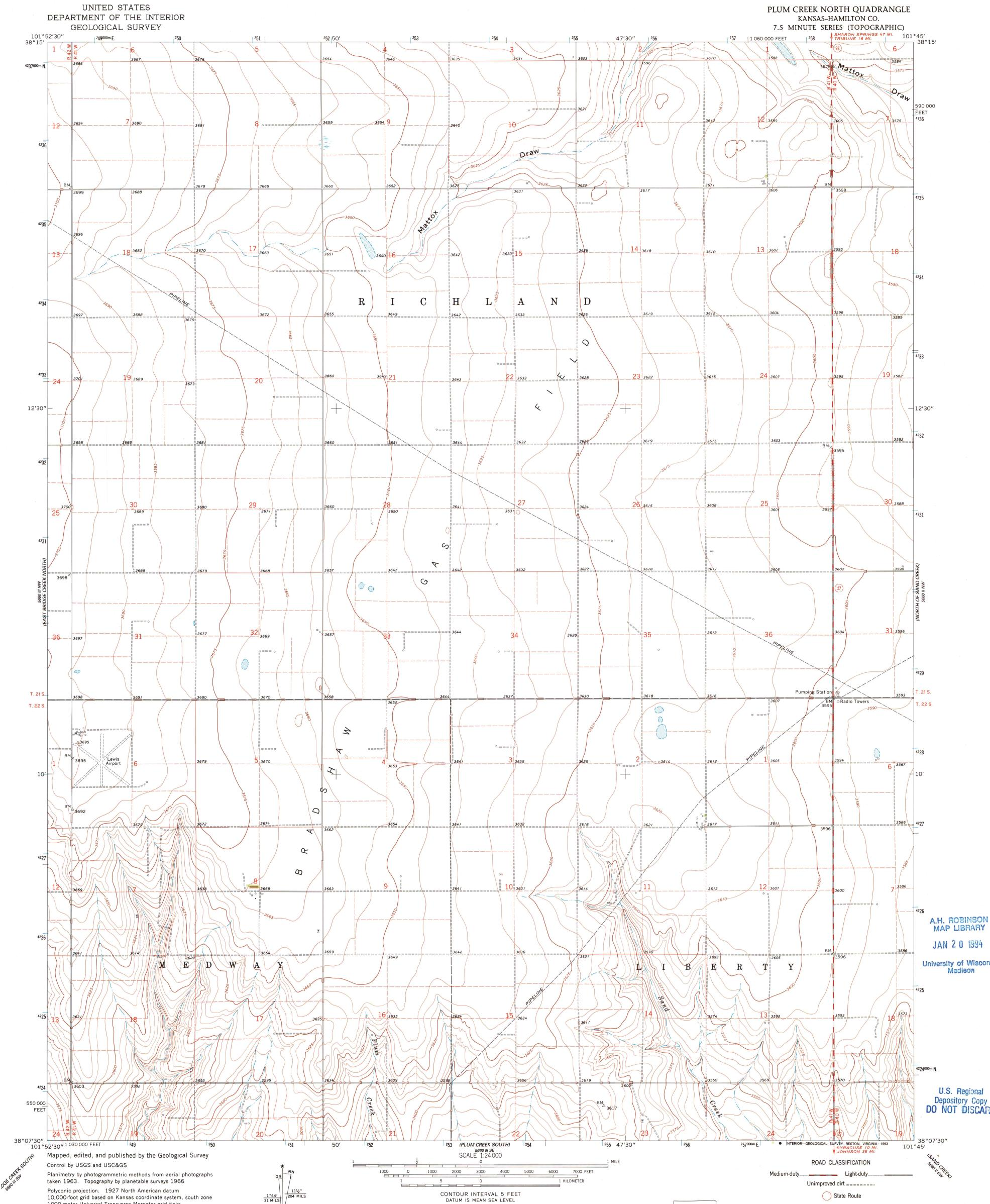
10,000-foot grid based on Kansas coordinate system, south zone 1000-meter Universal Transverse Mercator grid ticks, zone 14, shown in blue
