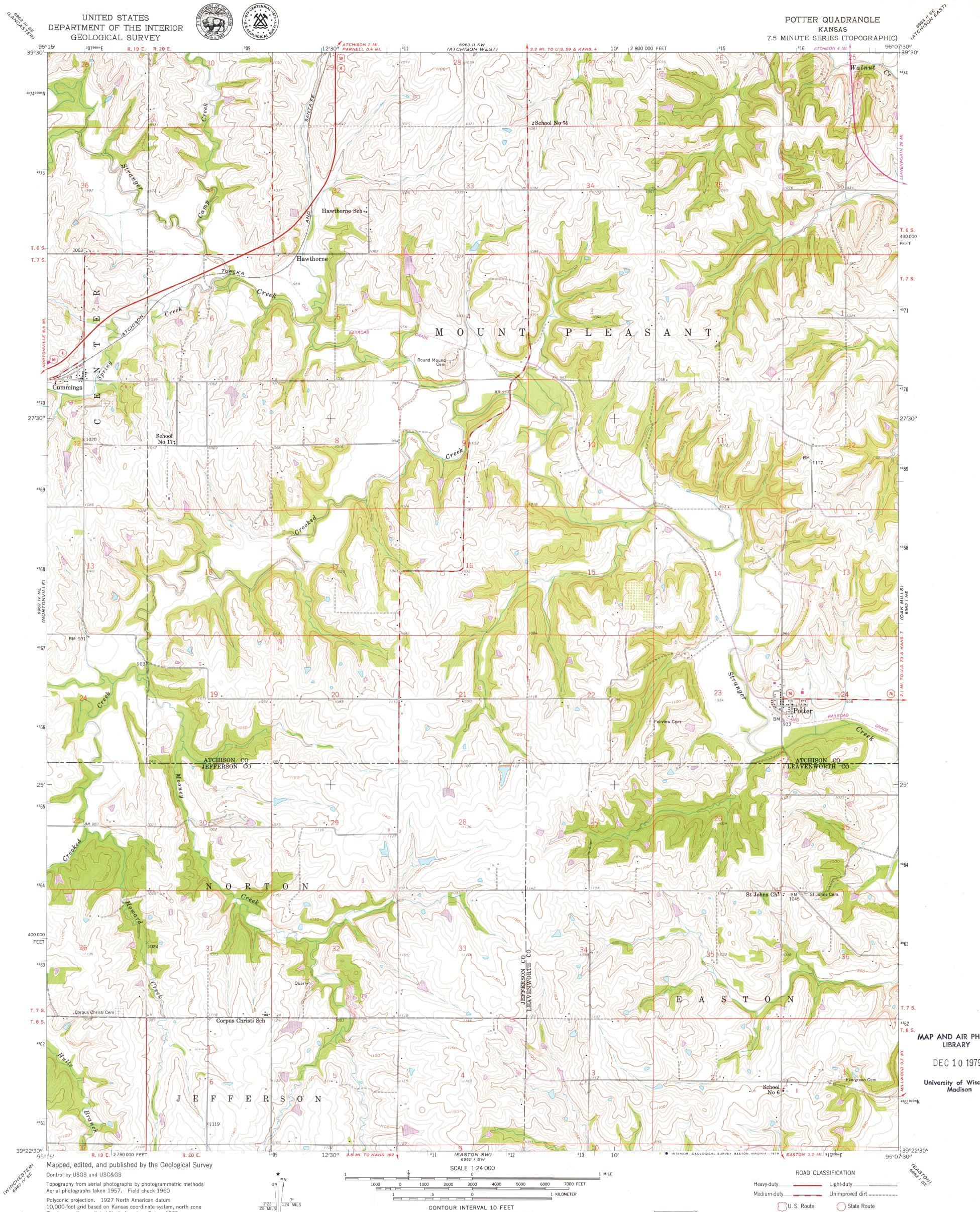
Polyconic projection. 1927 North American datum 10,000-foot grid based on Kansas coordinate system, north zone To place on the predicted North American Datum 1983 move the projection lines 3 meters north and 21 meters east as shown by dashed corner ticks 1000-meter Universal Transverse Mercator grid ticks, zone 15, shown in blue Revisions shown in purple compiled in cooperation with State of Kansas agencies from aerial photographs taken
