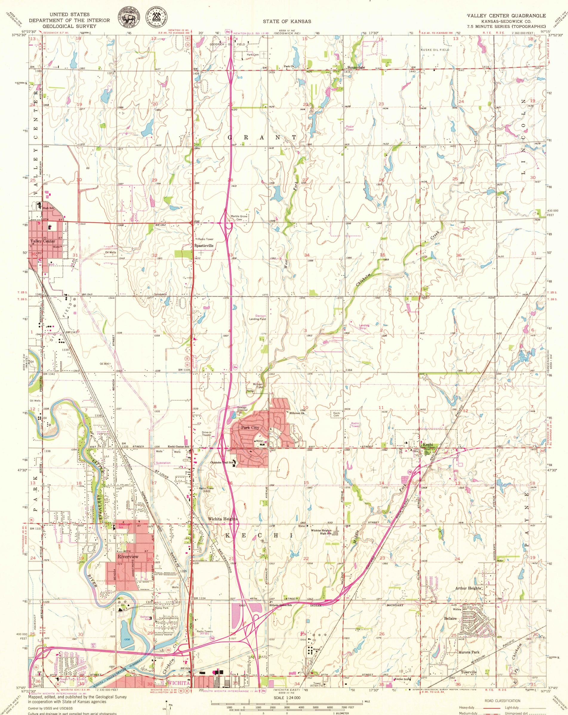
Culture and drainage in part compiled from aerial photographs taken 1954. Topography by planetable surveys 1939. Revised 1960 Polyconic projection. 1927 North American datum 10,000-foot grid based on Kansas coordinate system, south zone 1000-meter Universal Transverse Mercator grid ticks, zone 14, shown in blue UTM GRID AND 1970 MAGNETIC NORTH DECLINATION AT CENTER OF SHEET Red tint indicates areas in which only landmark buildings are shown
