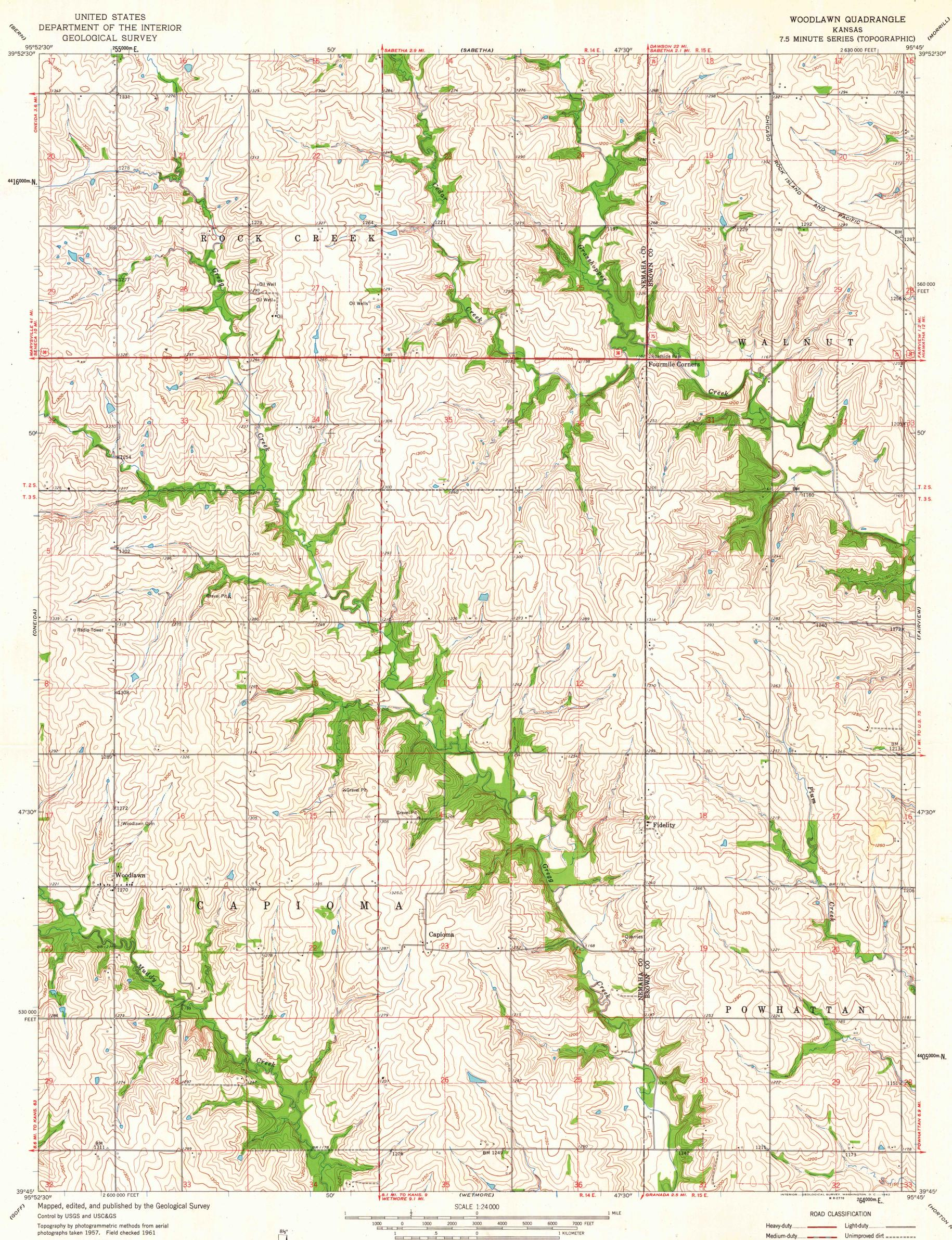
Polyconic projection. 1927 North American datum 10,000-foot grid based on Kansas coordinate system, north zone 1000-meter Universal Transverse Mercator grid ticks, zone 15, shown in blue Fine red dashed lines indicate selected fence and field lines where generally visible on aerial photographs. This information is unchecked
