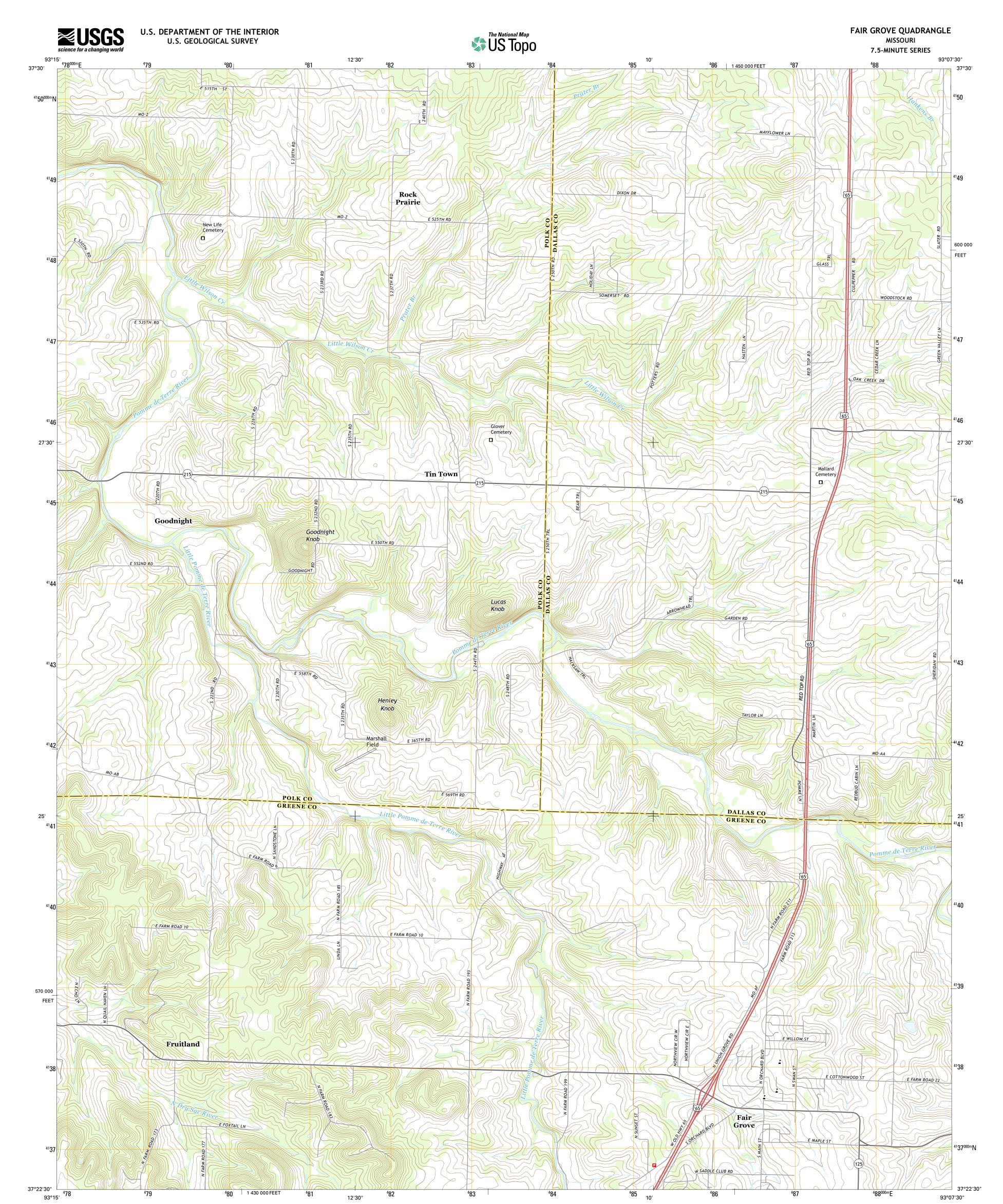
**Produced by the United States Geological Survey** North American Datum of 1983 (NAD83) World Geodetic System of 1984 (WGS84). Projection and 1 000-meter grid: Universal Transverse Mercator, Zone 15S 10 000-foot ticks: Missouri Coordinate System of 1983 (central zone)
