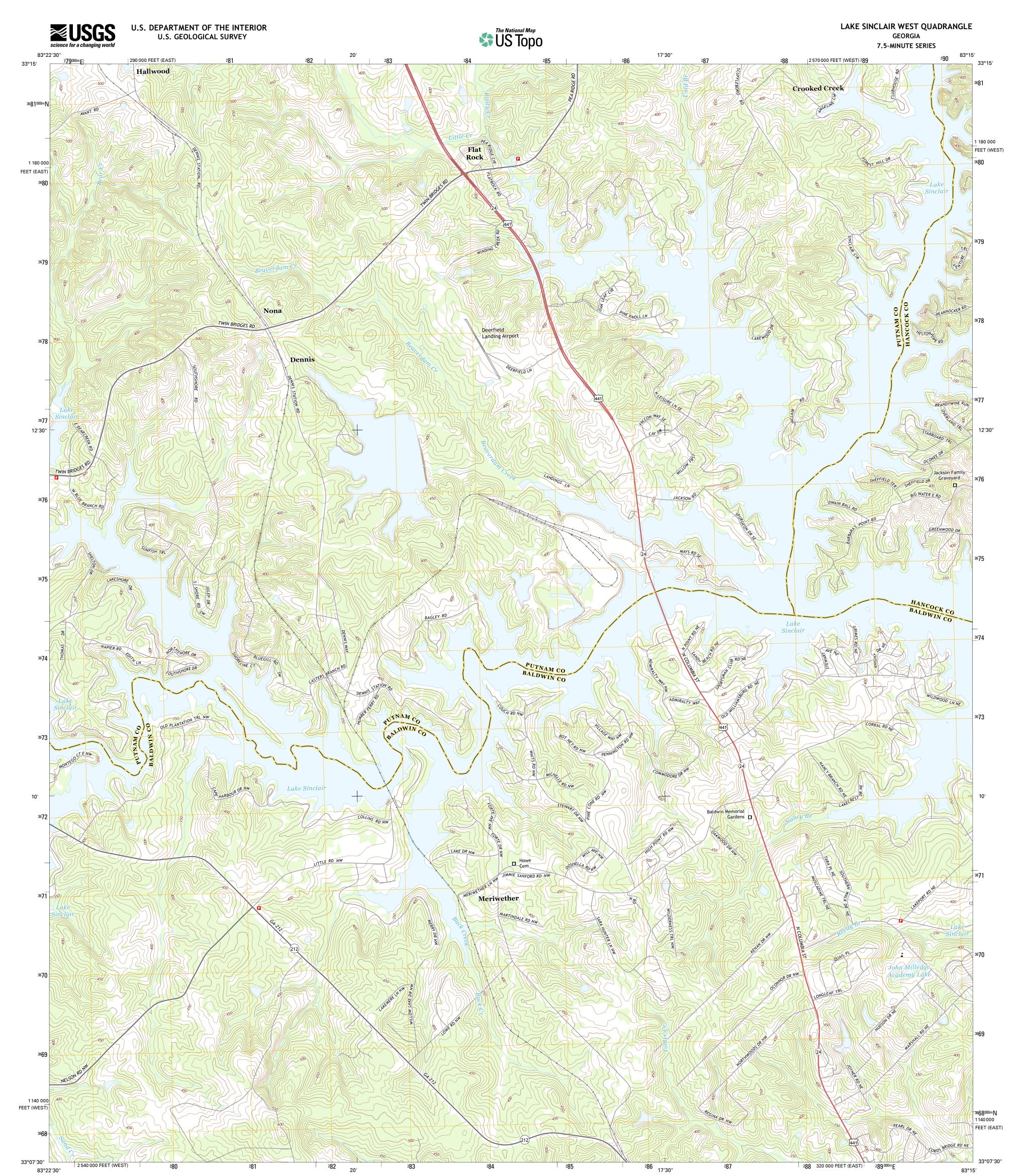
Produced by the United States Geological Survey North American Datum of 1983 (NAD83) World Geodetic System of 1984 (WGS84). Projection and 1 000-meter grid: Universal Transverse Mercator, Zone 17S 10 000-foot ticks: Georgia Coordinate System of 1983 (west and east zones)
