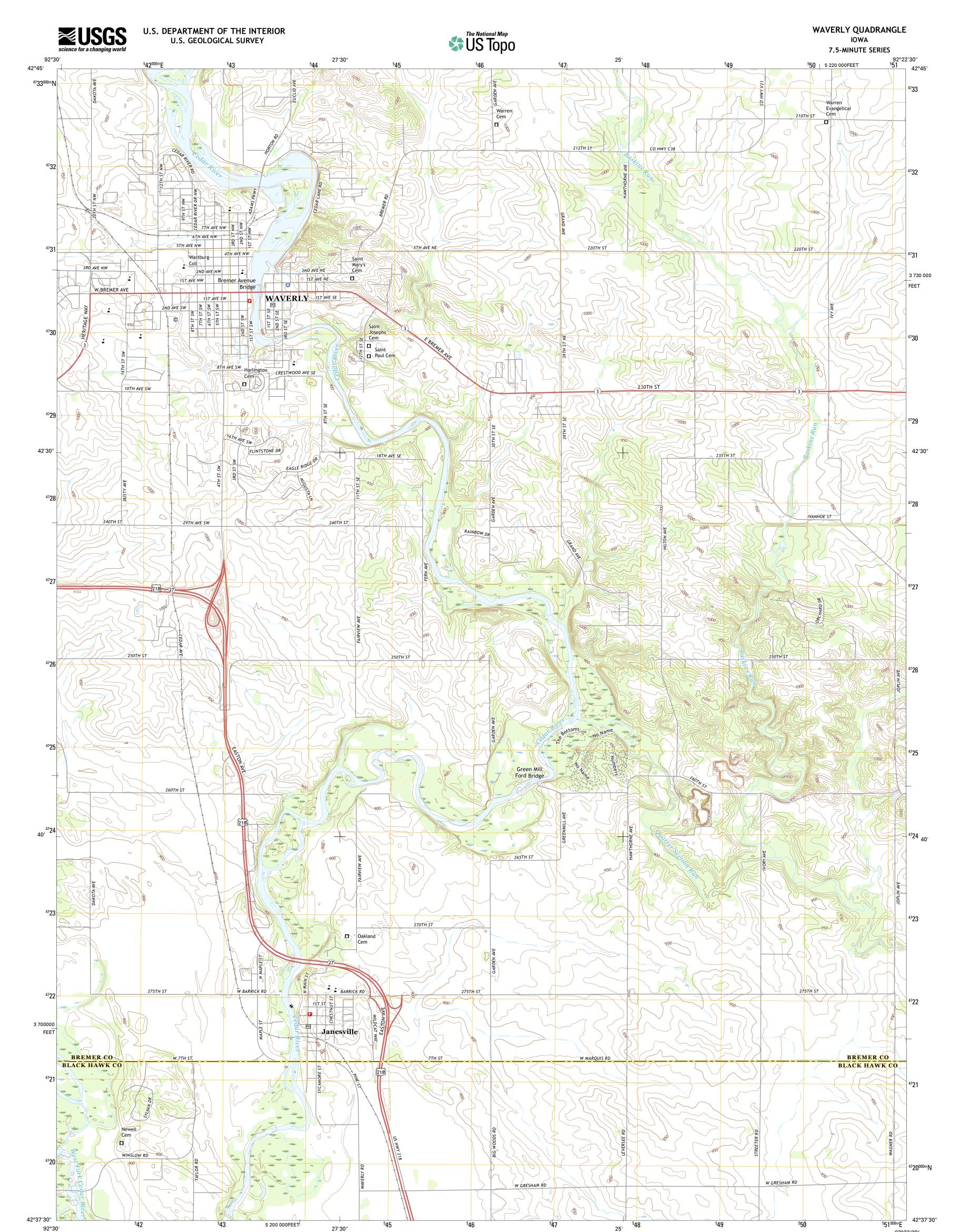
Produced by the United States Geological Survey North American Datum of 1983 (NAD83) World Geodetic System of 1984 (WGS84). Projection and 1 000-meter grid: Universal Transverse Mercator, Zone 15T 10 000-foot ticks: Iowa Coordinate System of 1983 (north zone) 0° 23 ′ 7 MILS
