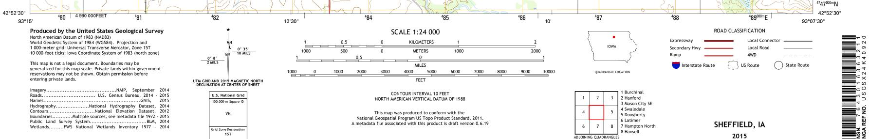
North American Datum of 1983 (NAD83) World Geodetic System of 1984 (WGS84). Projection and 1 000-meter grid: Universal Transverse Mercator, Zone 15T 10 000-foot ticks: Iowa Coordinate System of 1983 (north zone)
