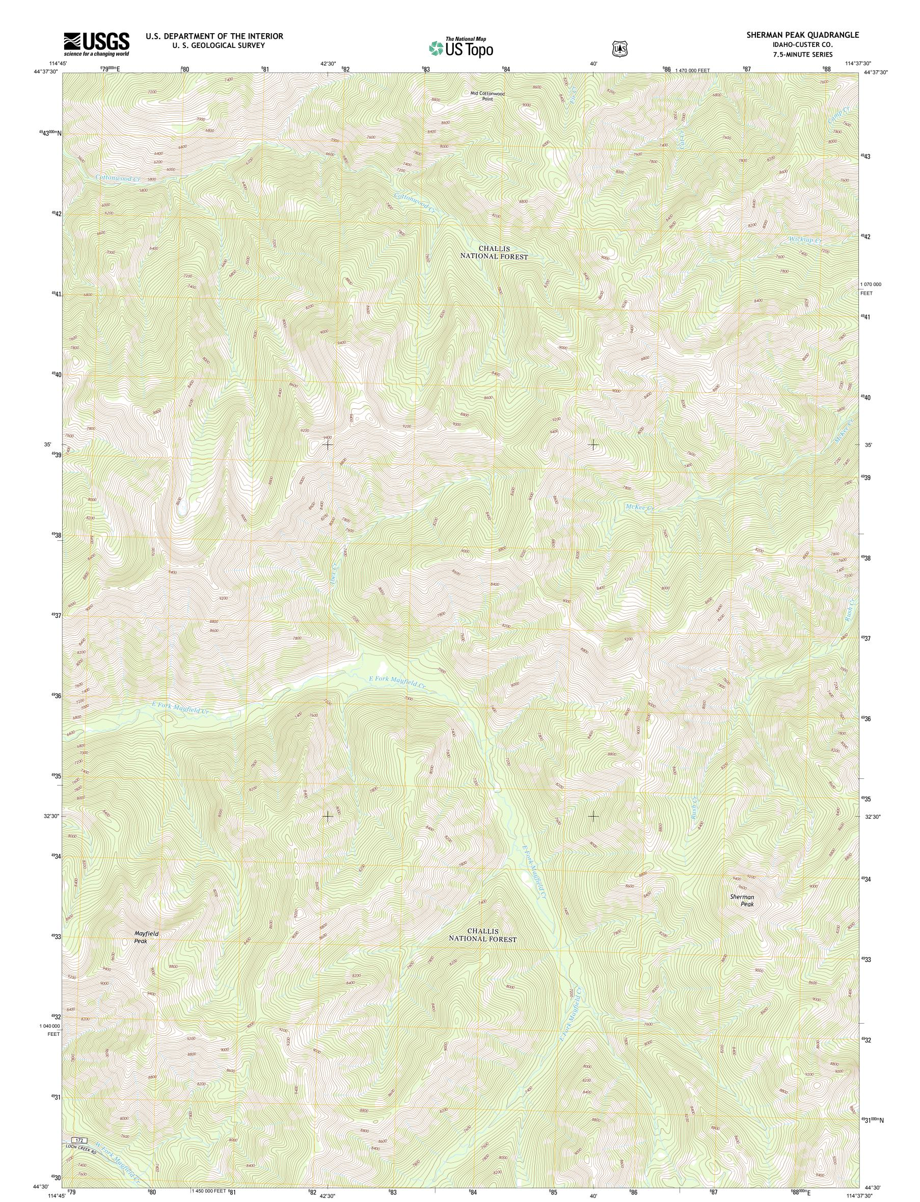
Produced by the United States Geological Survey North American Datum of 1983 (NAD83) World Geodetic System of 1984 (WGS84). Projection and 1 000-meter grid: Universal Transverse Mercator, Zone 11T 10 000-foot ticks: Idaho Coordinate System of 1983 (central zone)
