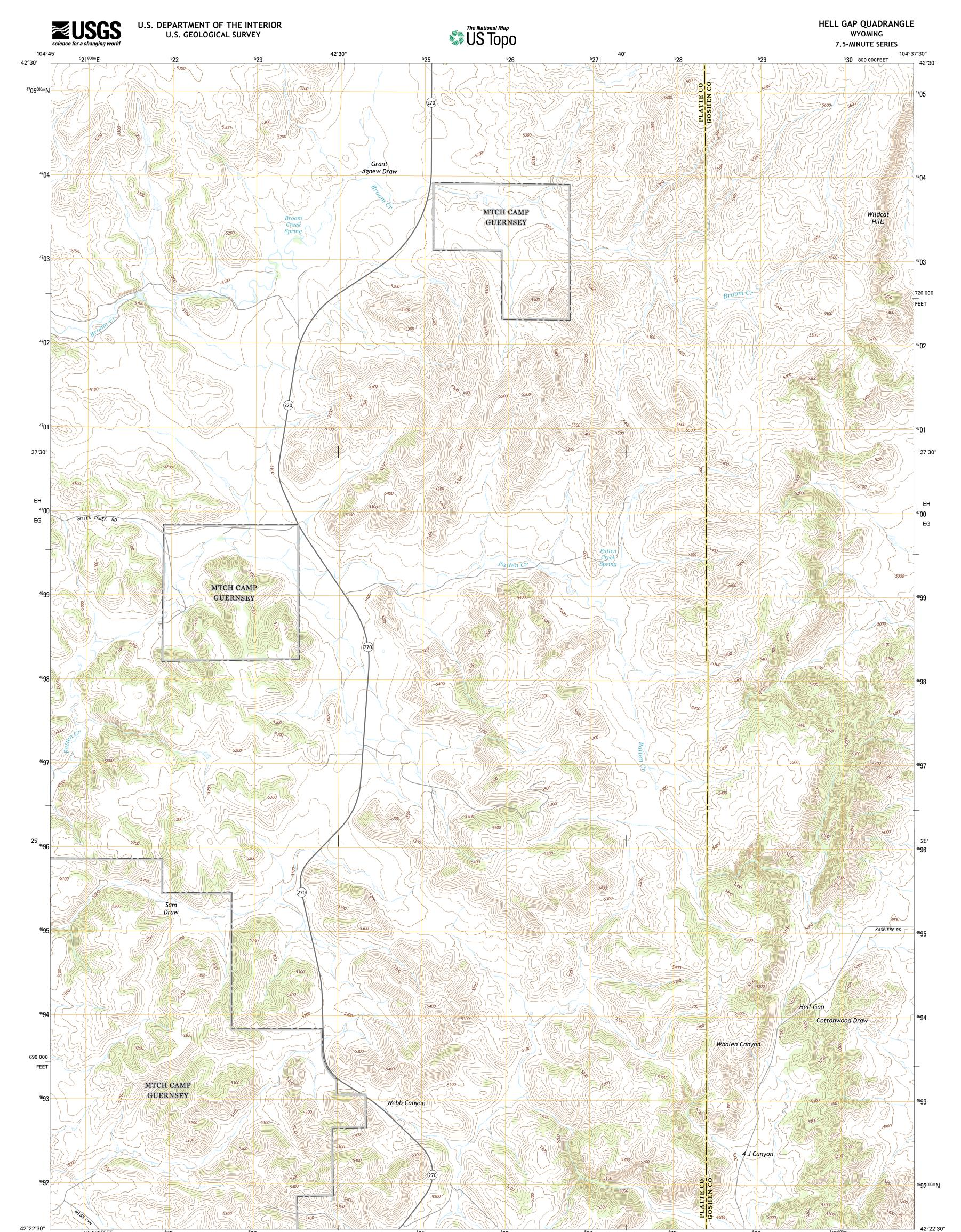
42°22'30" 770 000FEET <sup>5</sup>22 <sup>5</sup>23 ⁵**26** <sup>5</sup>25 104°45' 42'30" Produced by the United States Geological Survey North American Datum of 1983 (NAD83) World Geodetic System of 1984 (WGS84). Projection and 1 000-meter grid: Universal Transverse Mercator, Zone 13T 10 000-foot ticks: Wyoming Coordinate System of 1983 (east SCALE 1:24 000 KILOMETERS 0 <u>8° 36′</u> 153 MILS 500 METERS 1000 1000 0 zone) 0° 13′ 4 MILS
