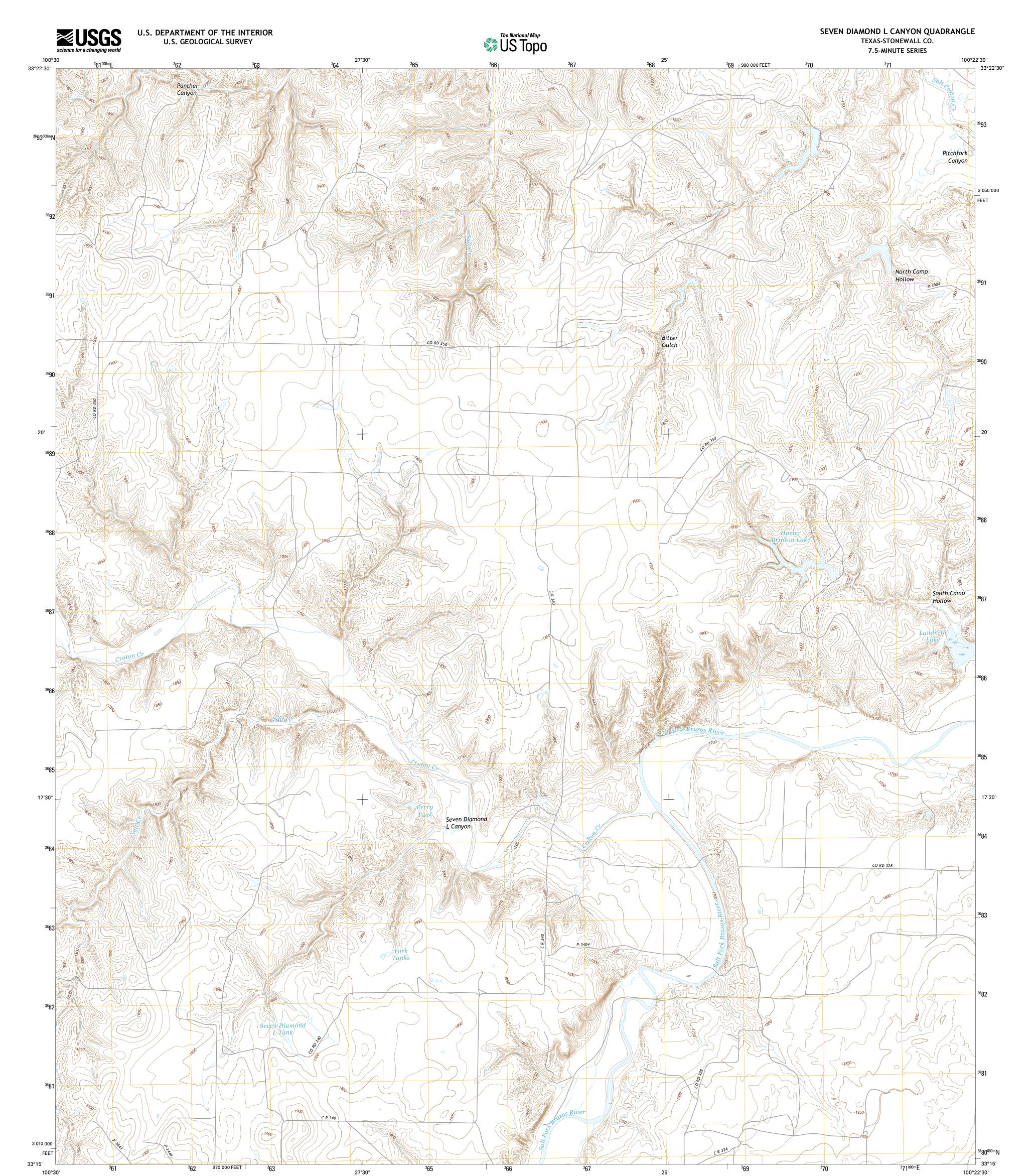
Produced by the United States Geological Survey North American Datum of 1983 (NAD83) World Geodetic System of 1984 (WGS84). Projection and 1 000-meter grid: Universal Transverse Mercator, Zone 14S 10 000-foot ticks: Texas Coordinate System of 1983 (north contral graph) central zone)
