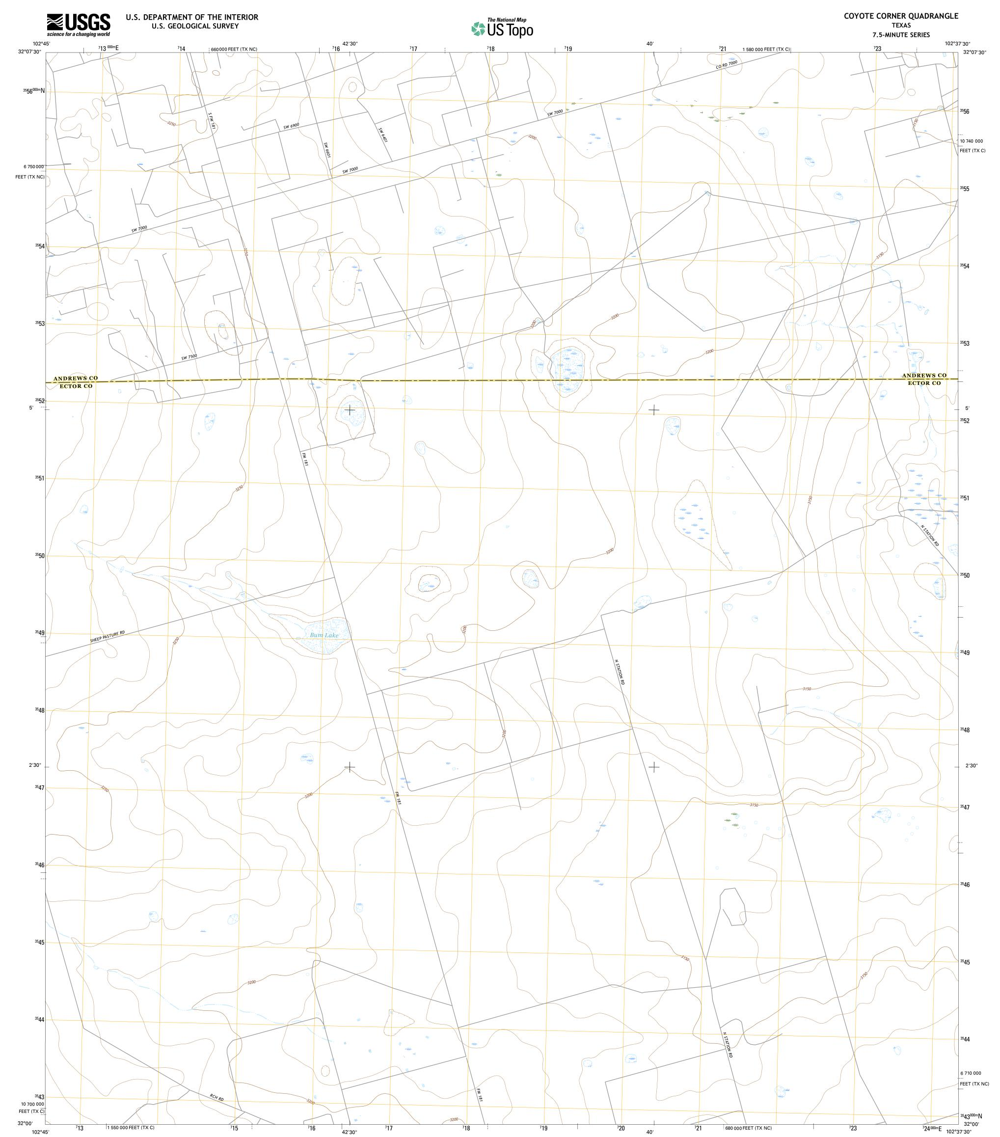
Produced by the United States Geological Survey North American Datum of 1983 (NAD83) World Geodetic System of 1984 (WGS84). Projection and 1 000-meter grid: Universal Transverse Mercator, Zone 13S 10 000-foot ticks: Texas Coordinate System of 1983 (central and north central zones)
