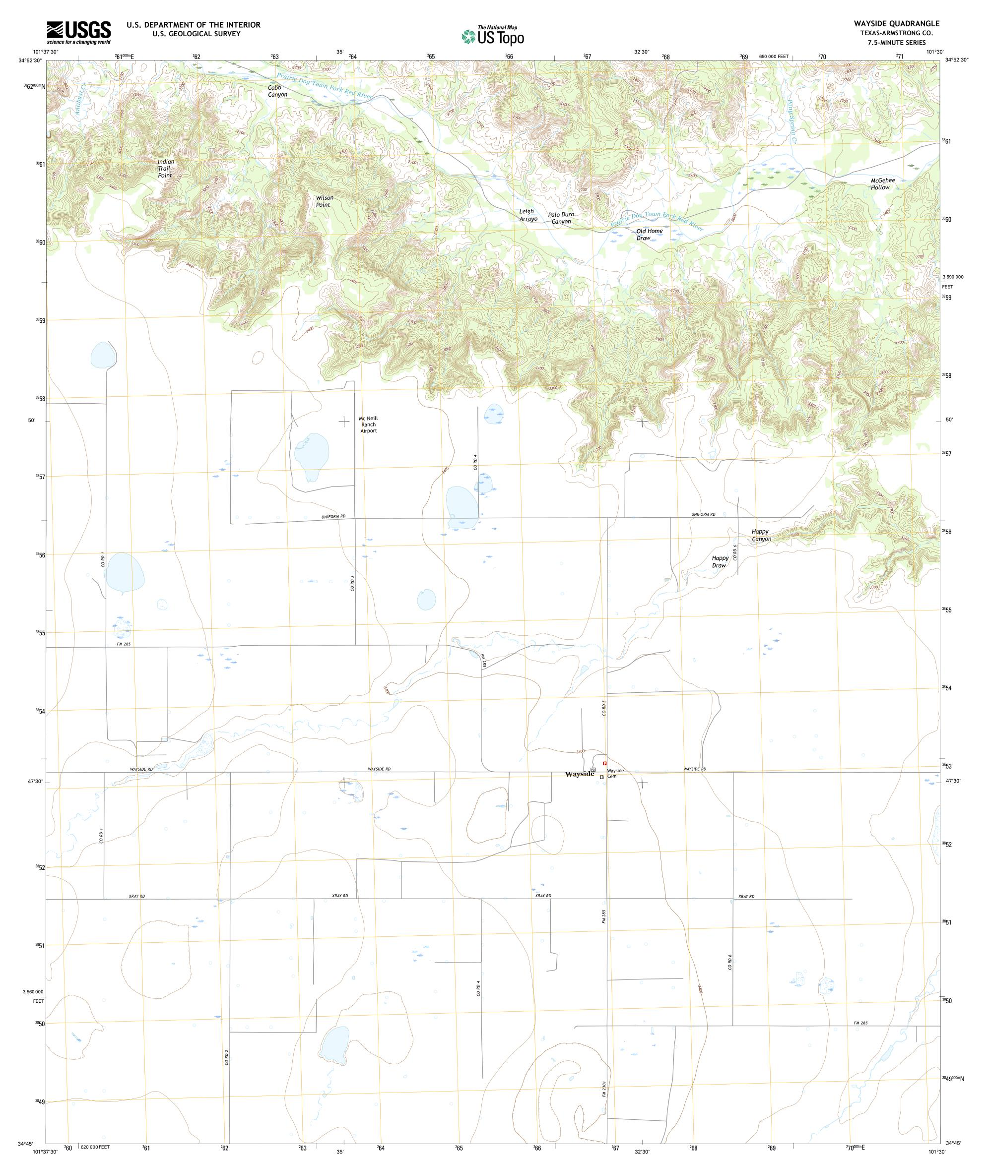
Produced by the United States Geological Survey North American Datum of 1983 (NAD83) World Geodetic System of 1984 (WGS84). Projection and 1 000-meter grid: Universal Transverse Mercator, Zone 14S 10 000-foot ticks: Texas Coordinate System of 1983 (north zone)
