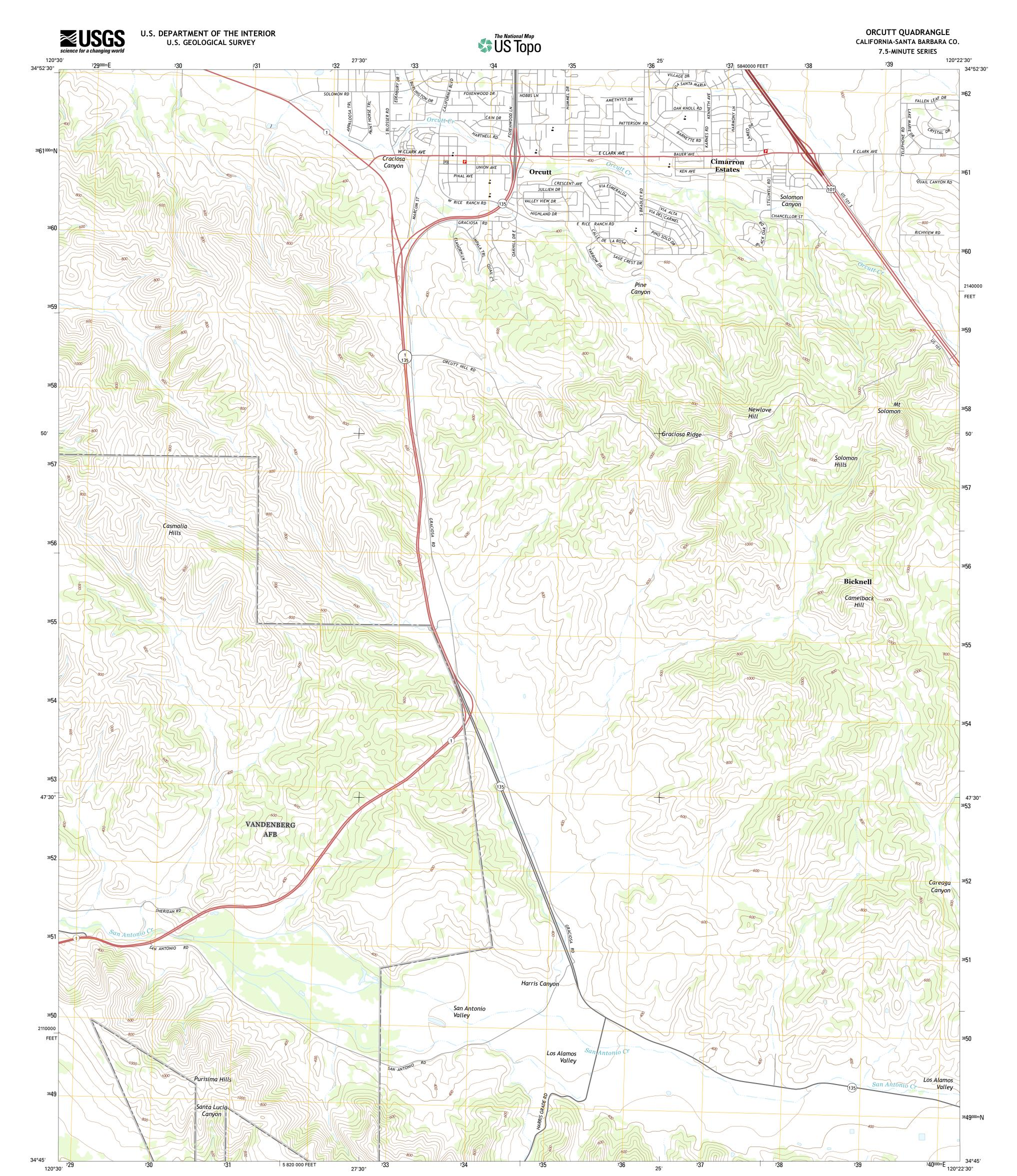
Produced by the United States Geological Survey North American Datum of 1983 (NAD83) World Geodetic System of 1984 (WGS84). Projection and 1 000-meter grid: Universal Transverse Mercator, Zone 10S 10 000-foot ticks: California Coordinate System of 1983 (zone 5)
