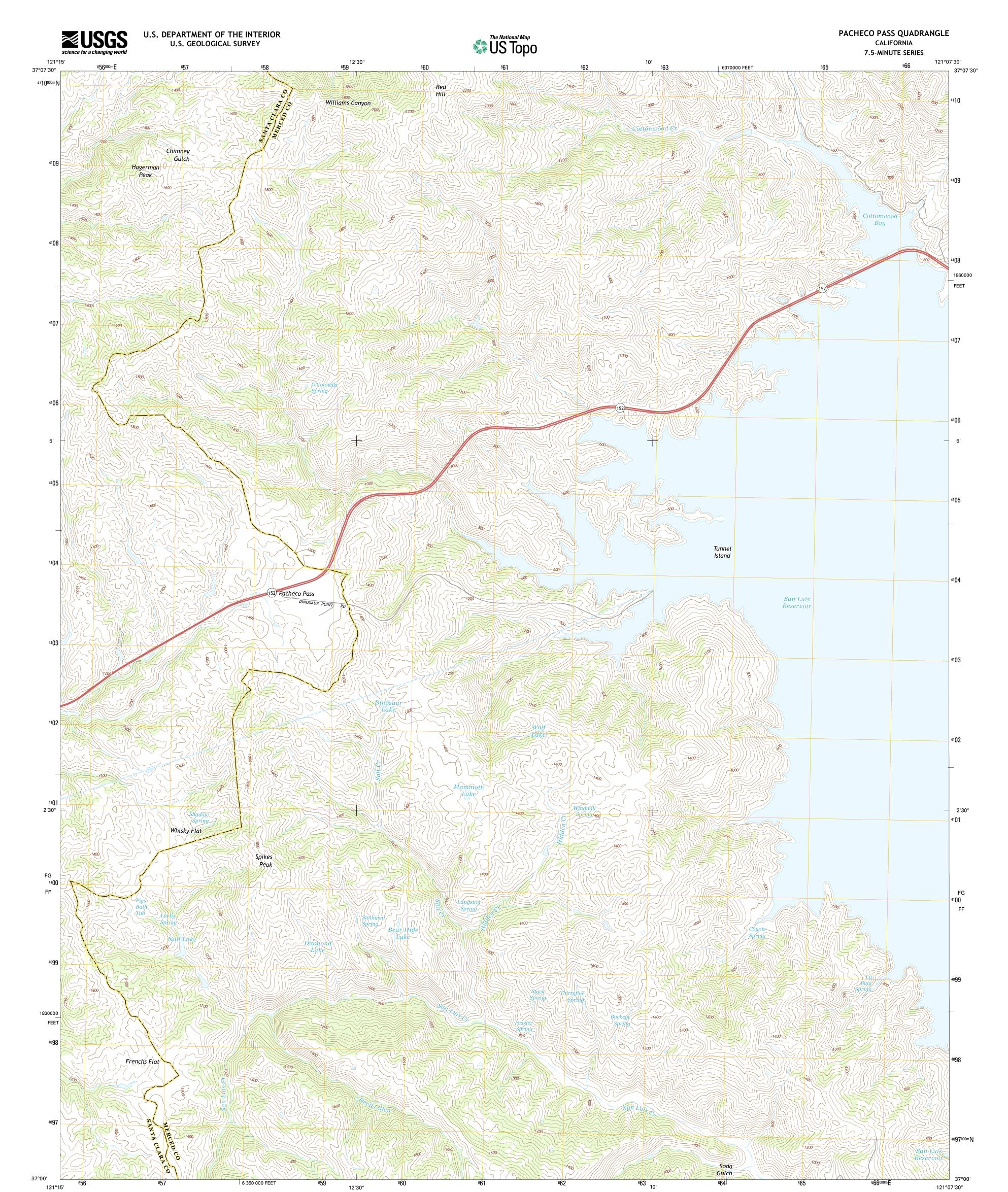
Produced by the United States Geological Survey North American Datum of 1983 (NAD83) World Geodetic System of 1984 (WGS84). Projection and 1 000-meter grid: Universal Transverse Mercator, Zone 10S 10 000-foot ticks: California Coordinate System of 1983 (zone 3)
