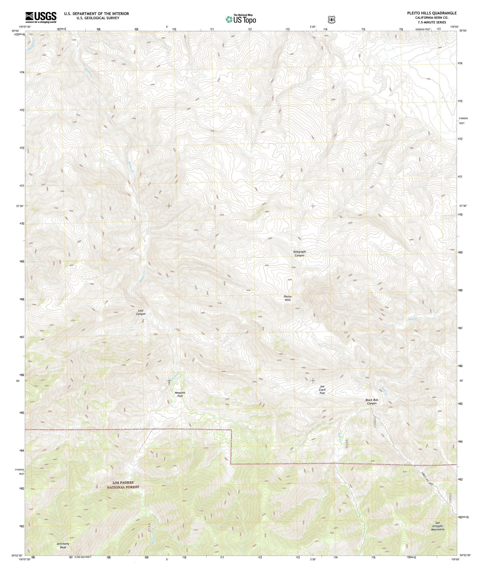
**Produced by the United States Geological Survey** North American Datum of 1983 (NAD83) World Geodetic System of 1984 (WGS84). Projection and 1 000-meter grid: Universal Transverse Mercator, Zone 11S 10 000-foot ticks: California Coordinate System of 1983 (zone 5)
