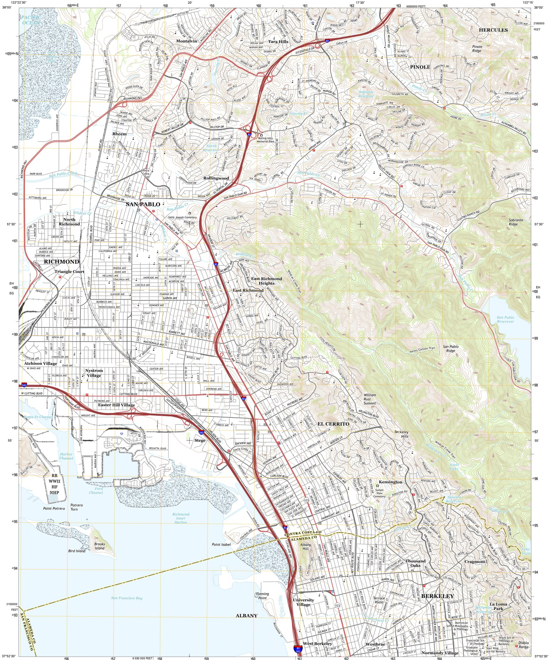
Produced by the United States Geological Survey North American Datum of 1983 (NAD83) World Geodetic System of 1984 (WGS84) Projection and 1 000-meter grid: Universal Transverse Mercator, Zone 10S 10 000-foot ticks: California Coordinate System of 1983 (zone 3) This map is not a legal document. Boundaries may be generalized for this map scale. Private lands within government reservations may not be shown. Obtain permission before entering private lands.
