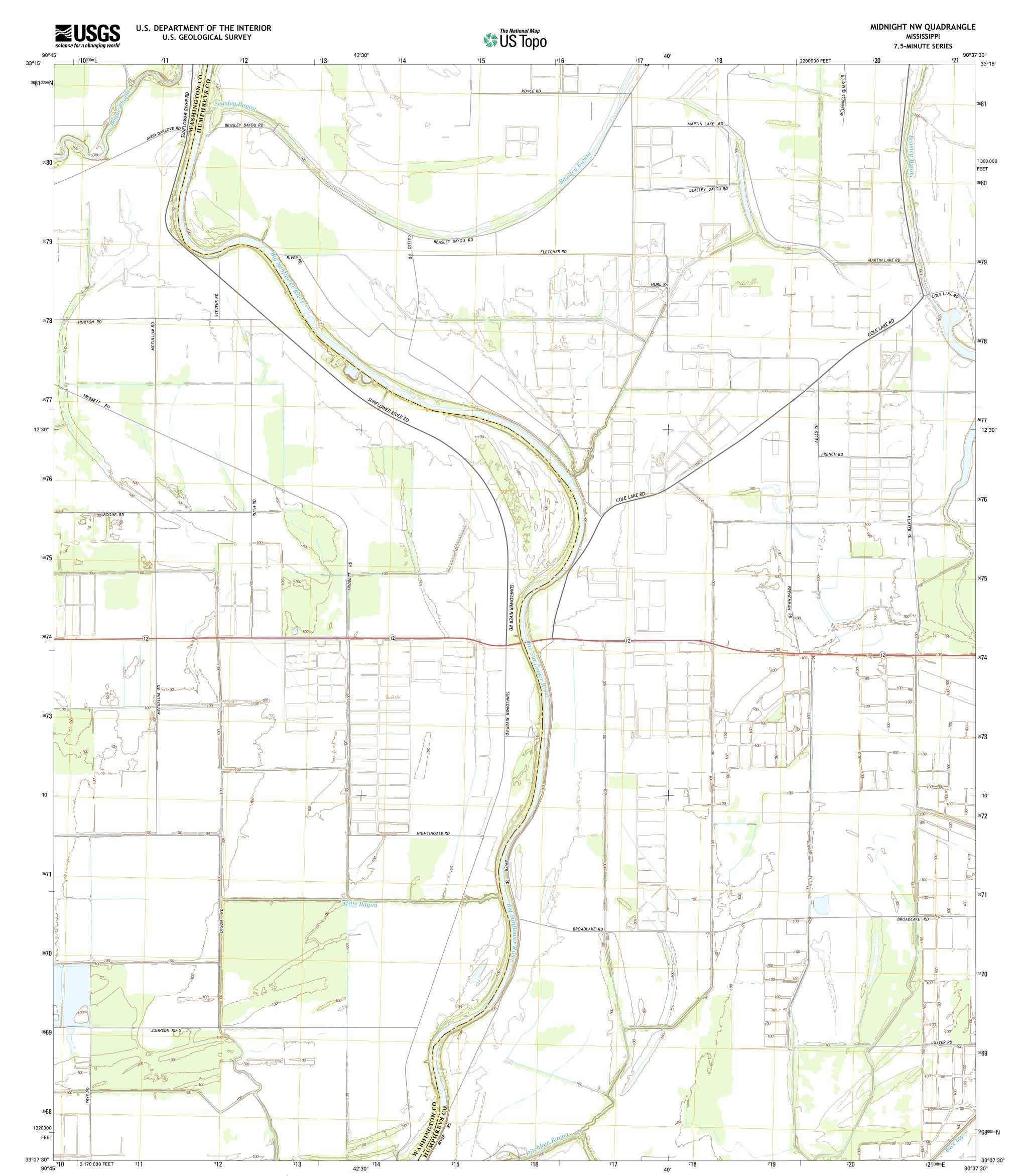
Produced by the United States Geological Survey North American Datum of 1983 (NAD83) World Geodetic System of 1984 (WGS84). Projection and 1 000-meter grid: Universal Transverse Mercator, Zone 15S 10 000-foot ticks: Mississippi Coordinate System of 1983 (west zone)
