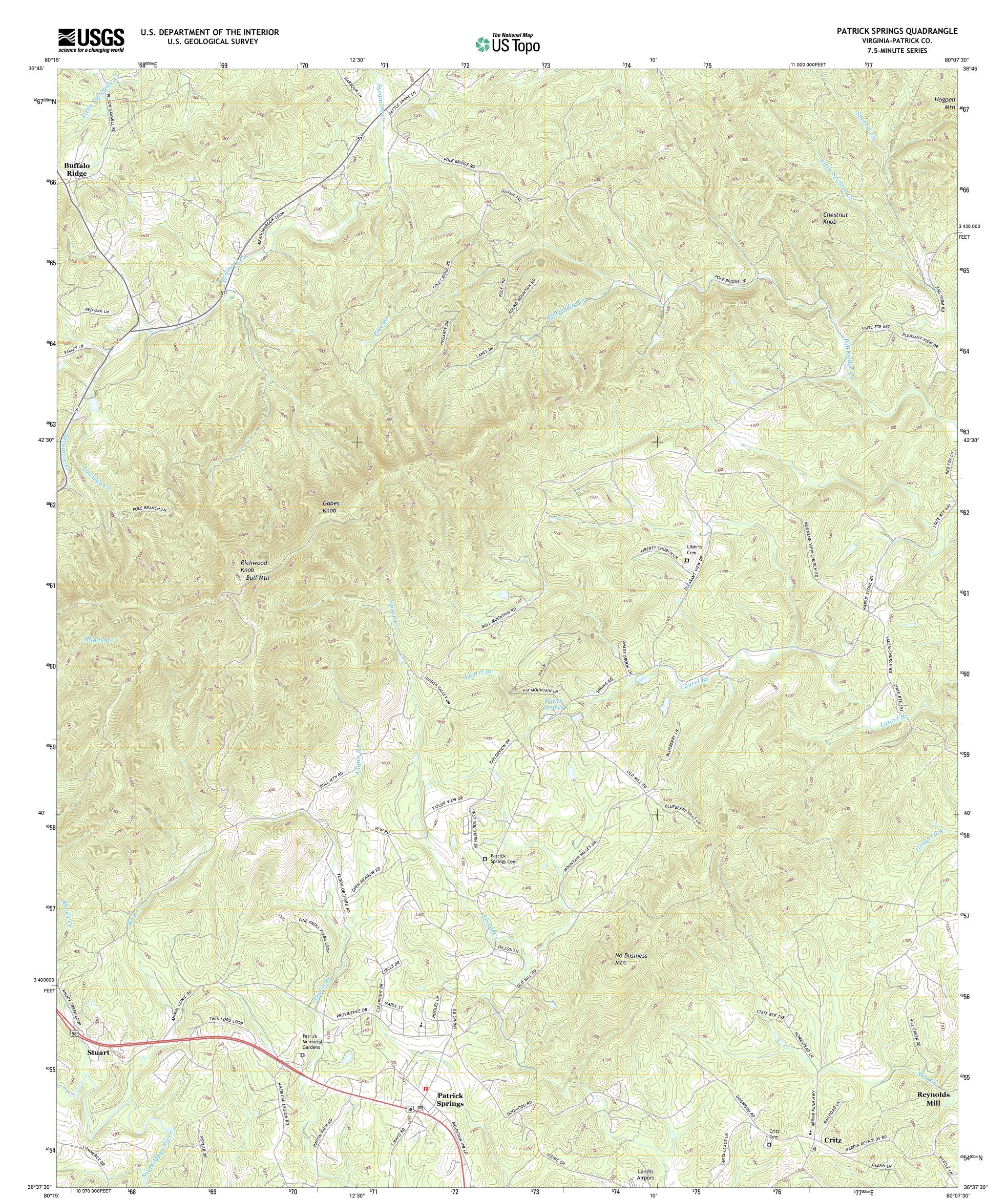
Produced by the United States Geological Survey North American Datum of 1983 (NAD83) World Geodetic System of 1984 (WGS84). Projection and 1 000-meter grid: Universal Transverse Mercator, Zone 17S 10 000-foot ticks: Virginia Coordinate System of 1983 (south zone)
