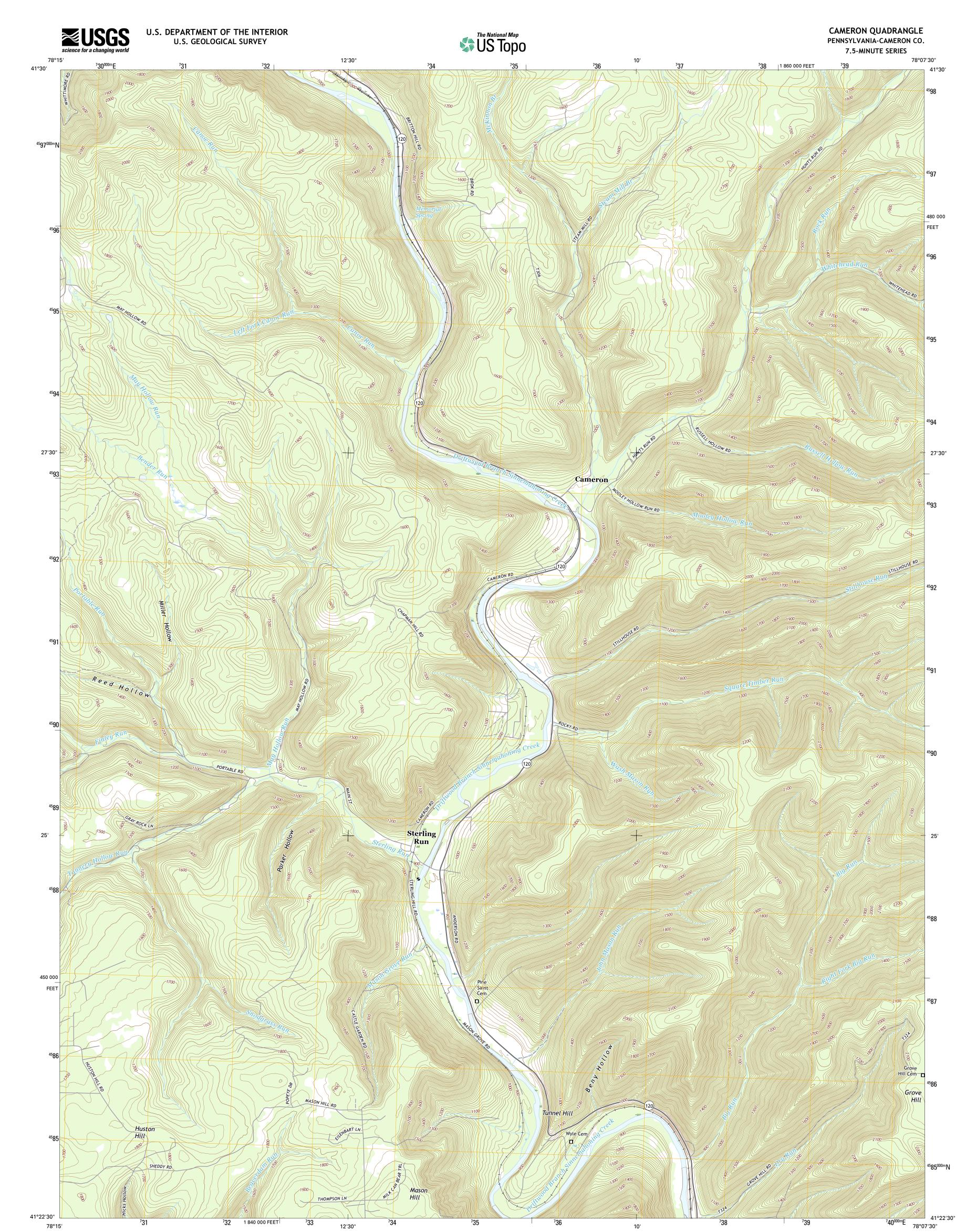
**Produced by the United States Geological Survey** North American Datum of 1983 (NAD83) World Geodetic System of 1984 (WGS84). Projection and 1 000-meter grid: Universal Transverse Mercator, Zone 17T 10 000-foot ticks: Pennsylvania Coordinate System of 1983 (north zone) (north zone)
