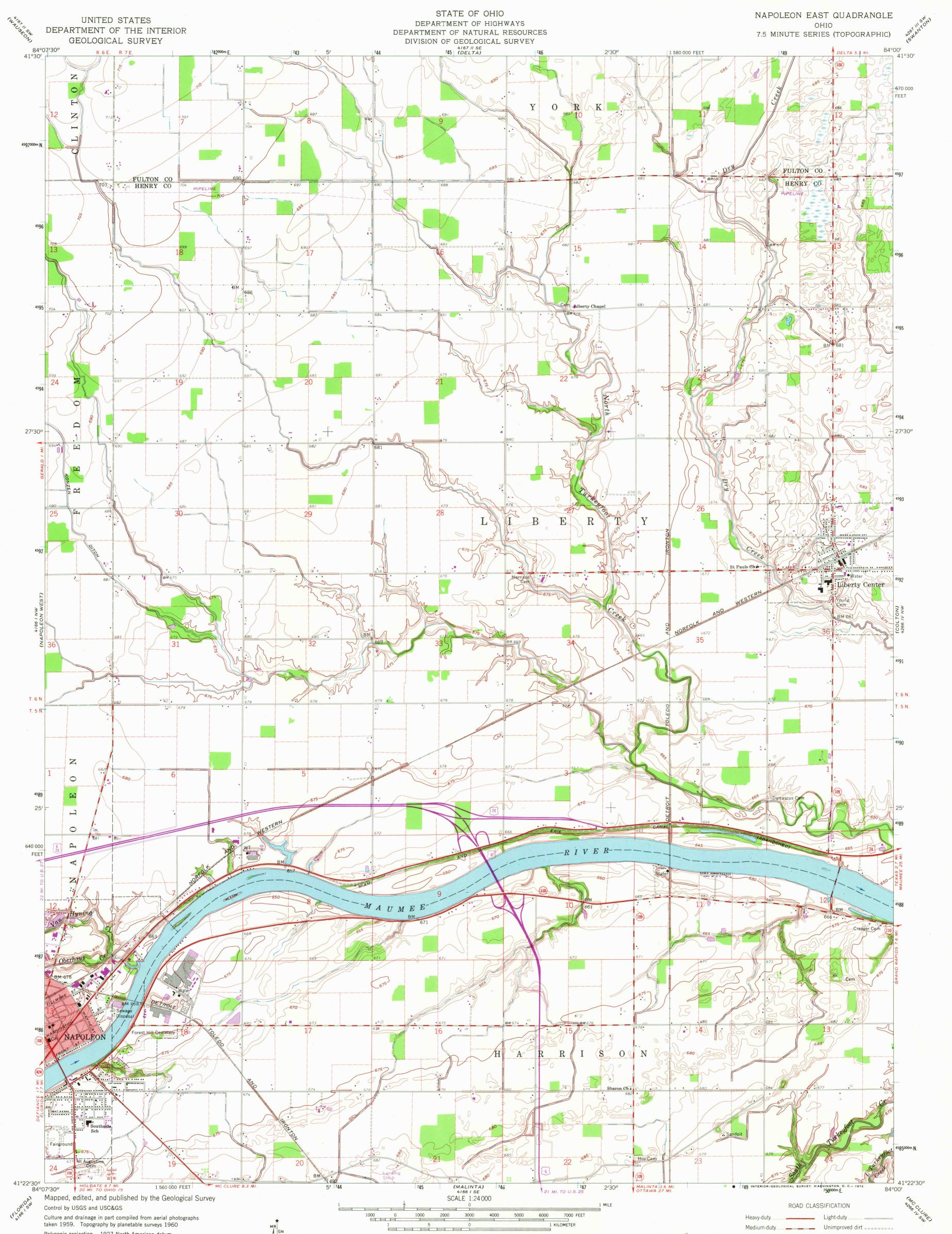
Polyconic projection. 1927 North American datum 10,000-foot grid based on Ohio coordinate system, north zone 1000-meter Universal Transverse Mercator grid ticks, zone 16, shown in blue
