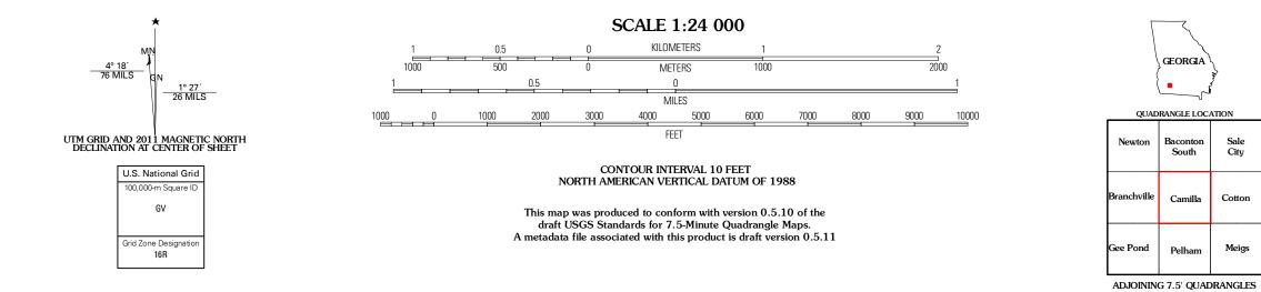
Produced by the United States Geological Survey North American Datum of 1983 (NAD83) World Geodetic System of 1984 (WGS84). Projection and 1 000-meter grid: Universal Transverse Mercator, Zone 16R 10 000-foot ticks: Georgia Coordinate System of 1983 (west zone)
