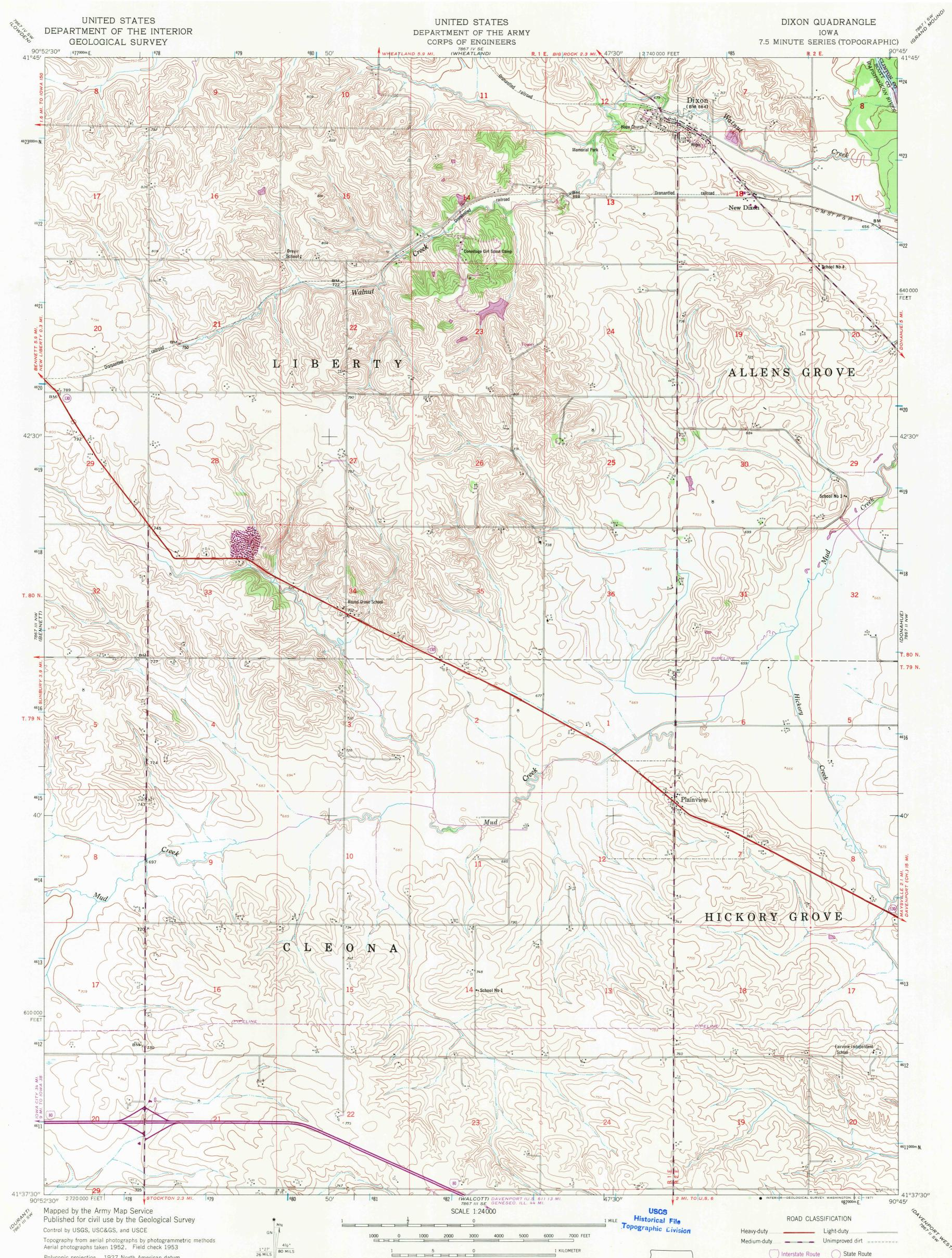
Polyconic projection. 1927 North American datum 10,000-foot grid based on Iowa coordinate system, south zone 1000-meter Universal Transverse Mercator grid ticks, zone 15, shown in blue Unchecked elevations are shown in brown
