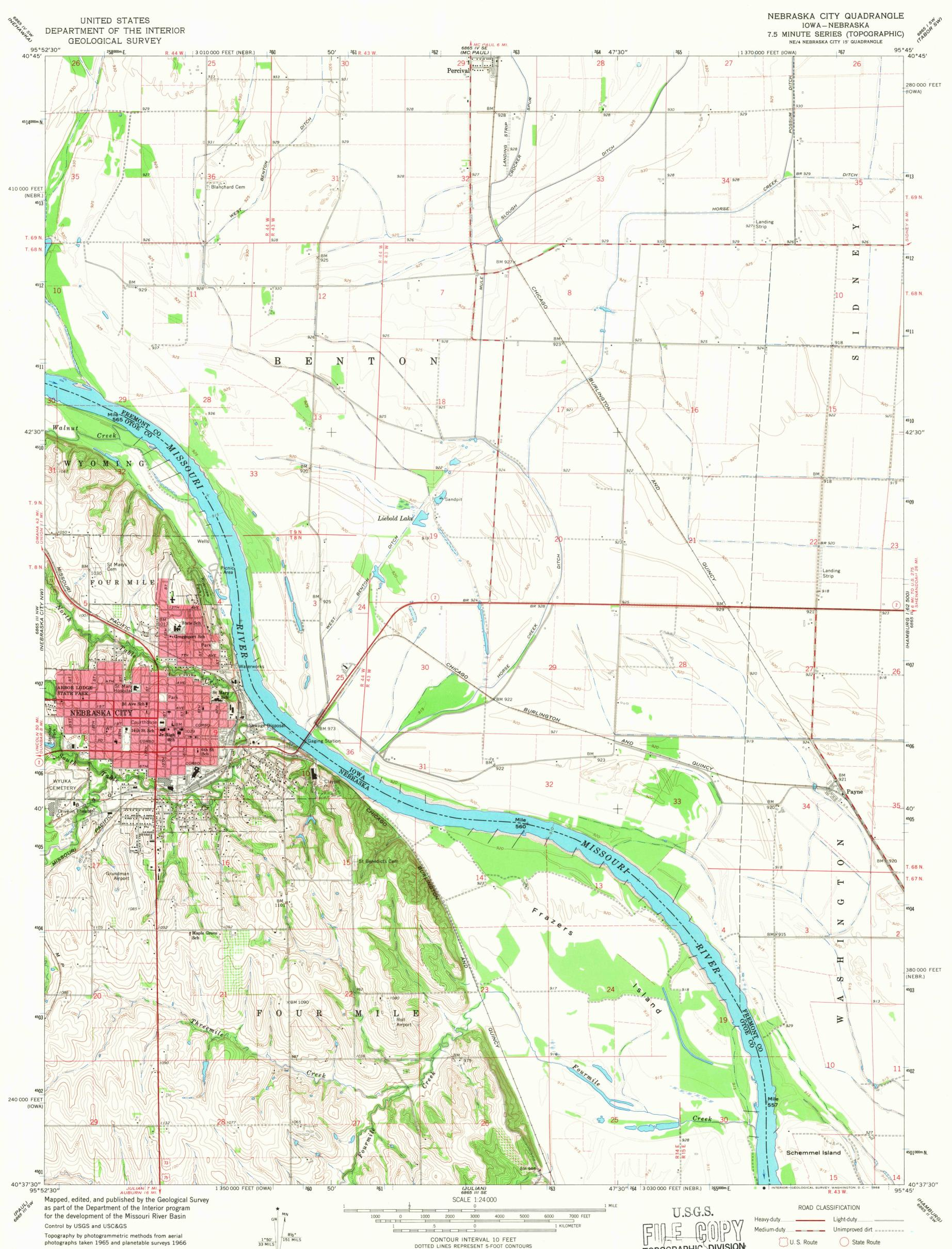
Topography by photogrammetric methods from aerial photographs taken 1965 and planetable surveys 1966 Polyconic projection. 1927 North American datum
