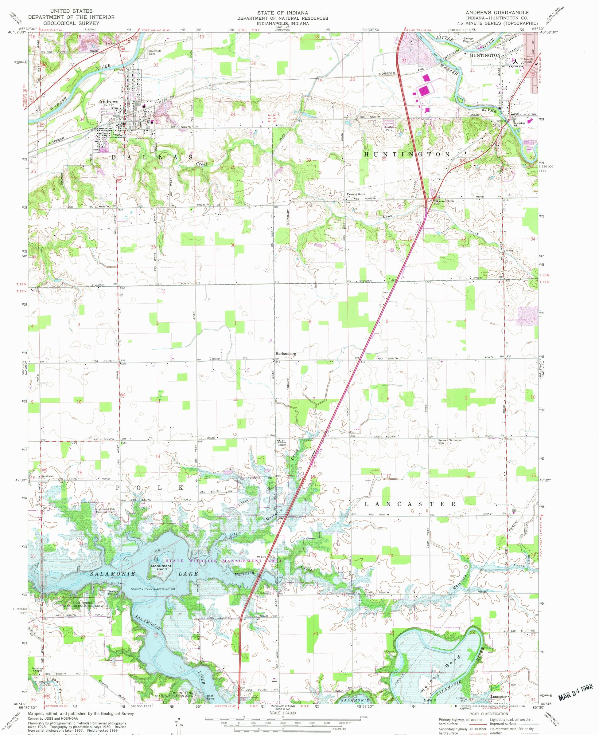
Polyconic projection. 10,000-foot grid ticks based on Indiana coordinate system, east zone. 1000-meter Universal Transverse Mercator grid ticks, zone 16, shown in blue. 1927 North American Datum. To place on the predicted North American Datum 1983 move the projection lines 1 meter south and 2 meters west as shown by dashed corner ticks
