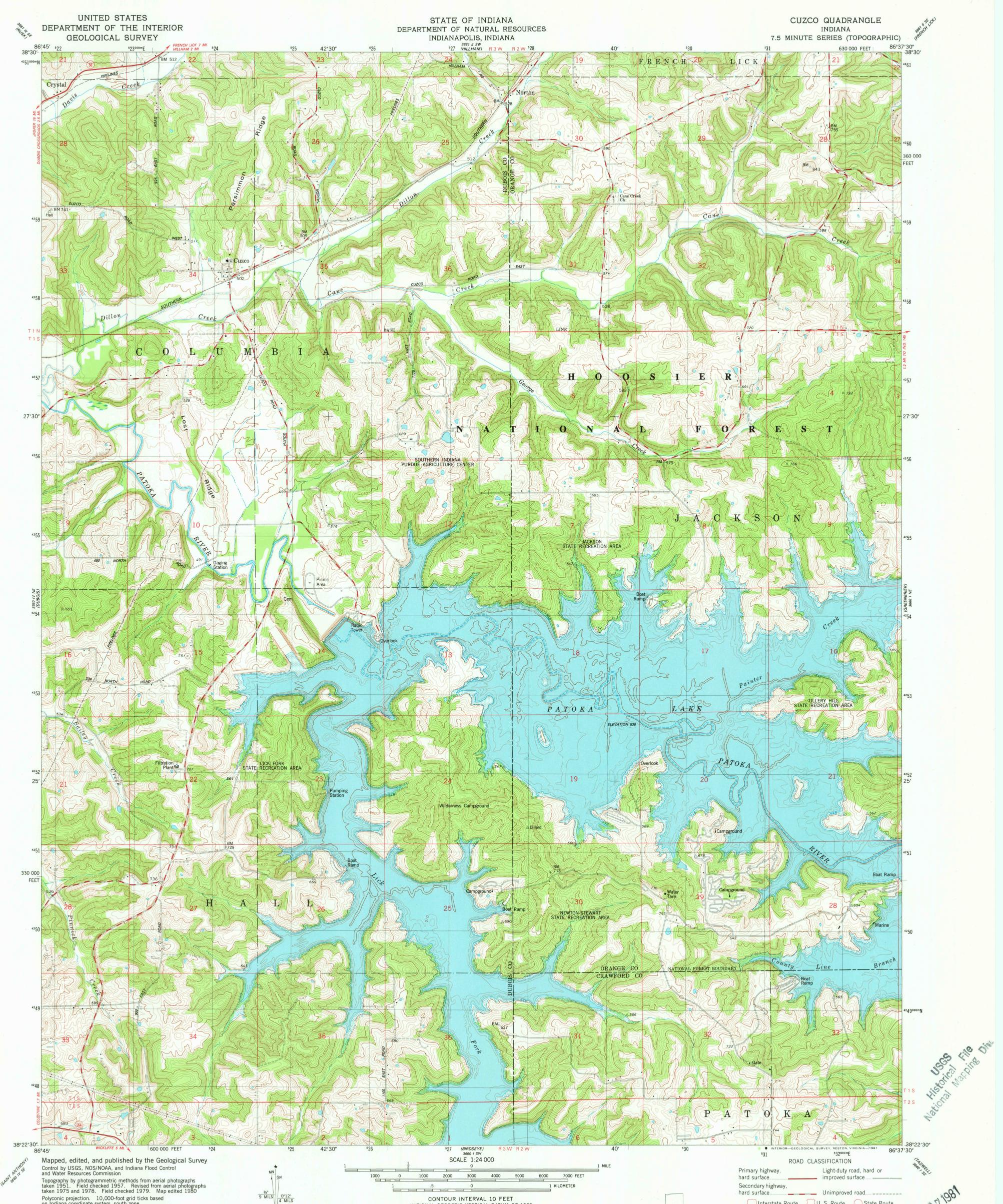
Polyconic projection. 10,000-foot grid ticks based on Indiana coordinate system, south zone 1000-meter Universal Transverse Mercator grid, zone 16 1927 North American Datum To place on the predicted North American Datum 1983 move the projection lines 3 meters south as shown by dashed corner ticks
