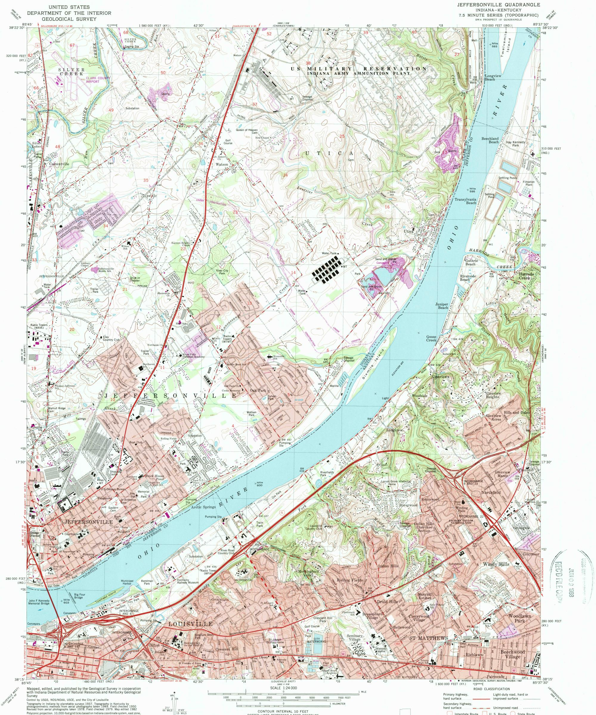
Polyconic projection. 10,000-foot grid ticks based on Indiana coordinate system, east zone, and Kentucky coordinate system, north zone 1000-meter Universal Transverse Mercator grid, zone 16. 1927 North American Datum To place on the predicted North American Datum 1983 move the projection lines 3 meters south and 3 meters west as shown by dashed corner ticks Fine red dashed lines indicate selected fence and field lines where visible on aerial photographs. This information is unchecked
