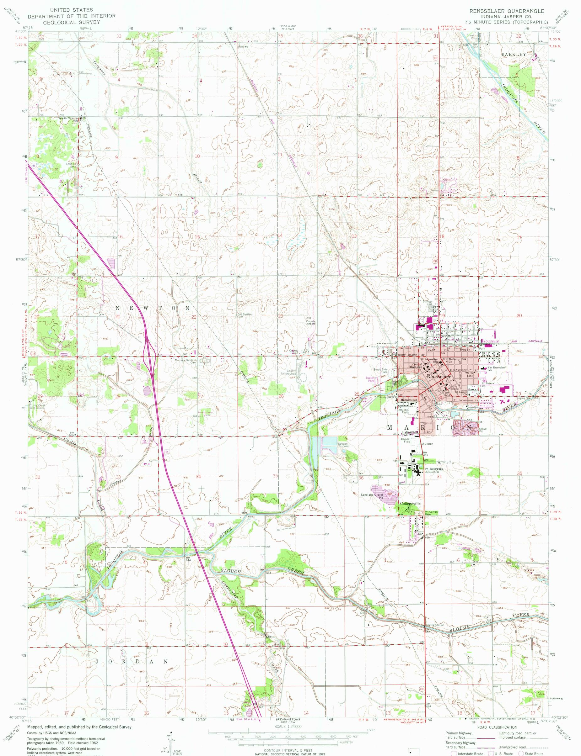
Indiana coordinate system, west zone 1000-meter Universal Transverse Mercator grid ticks, zone 16, shown in blue. 1927 North American Datum To place on the predicted North American Datum 1983 move the projection lines 3 meters east as shown by dashed corner ticks
