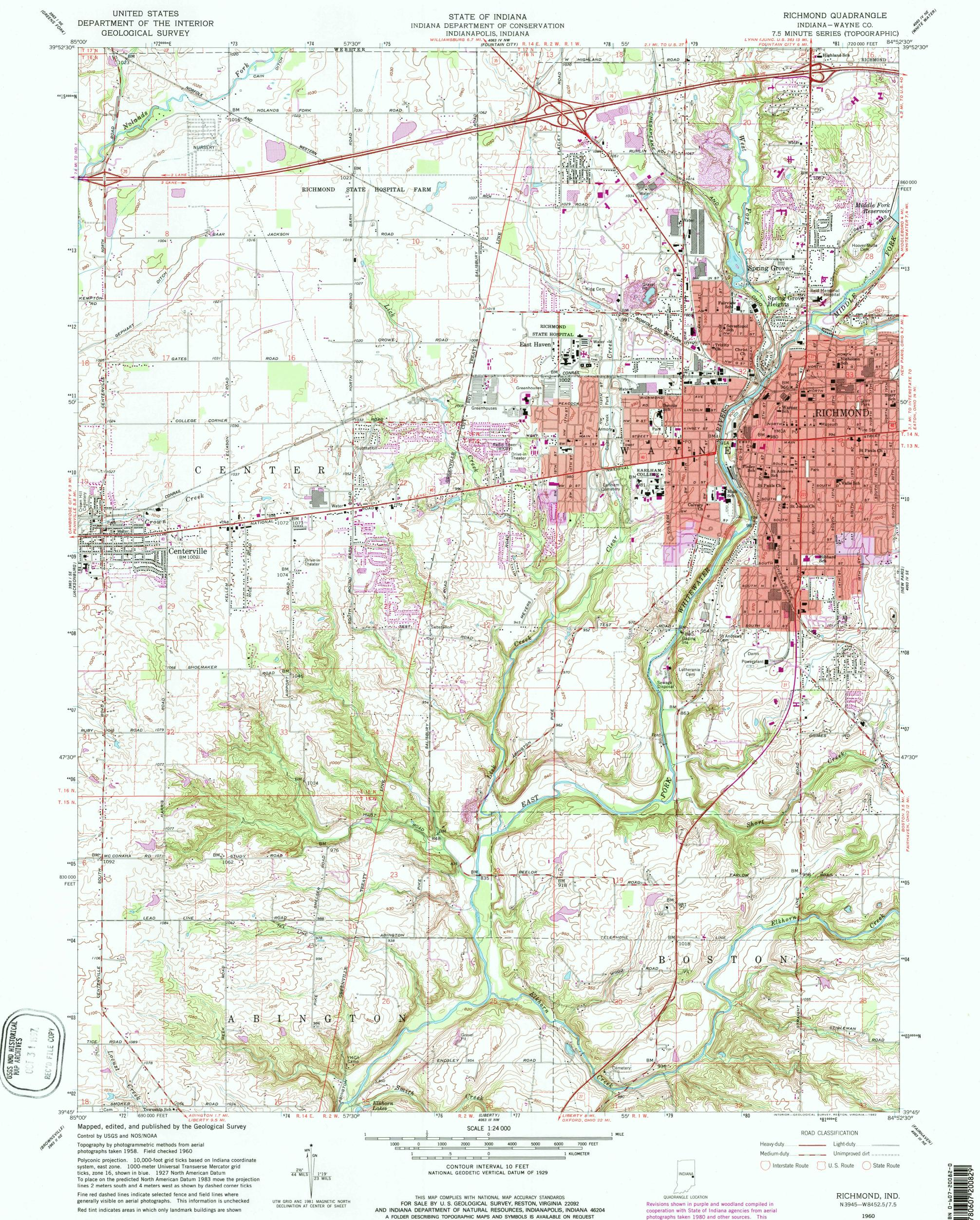
Polyconic projection. 10,000-foot grid ticks based on Indiana coordinate system, east zone. 1000-meter Universal Transverse Mercator grid ticks, zone 16, shown in blue. 1927 North American Datum To place on the predicted North American Datum 1983 move the projection lines 2 meters south and 4 meters west as shown by dashed corner ticks
