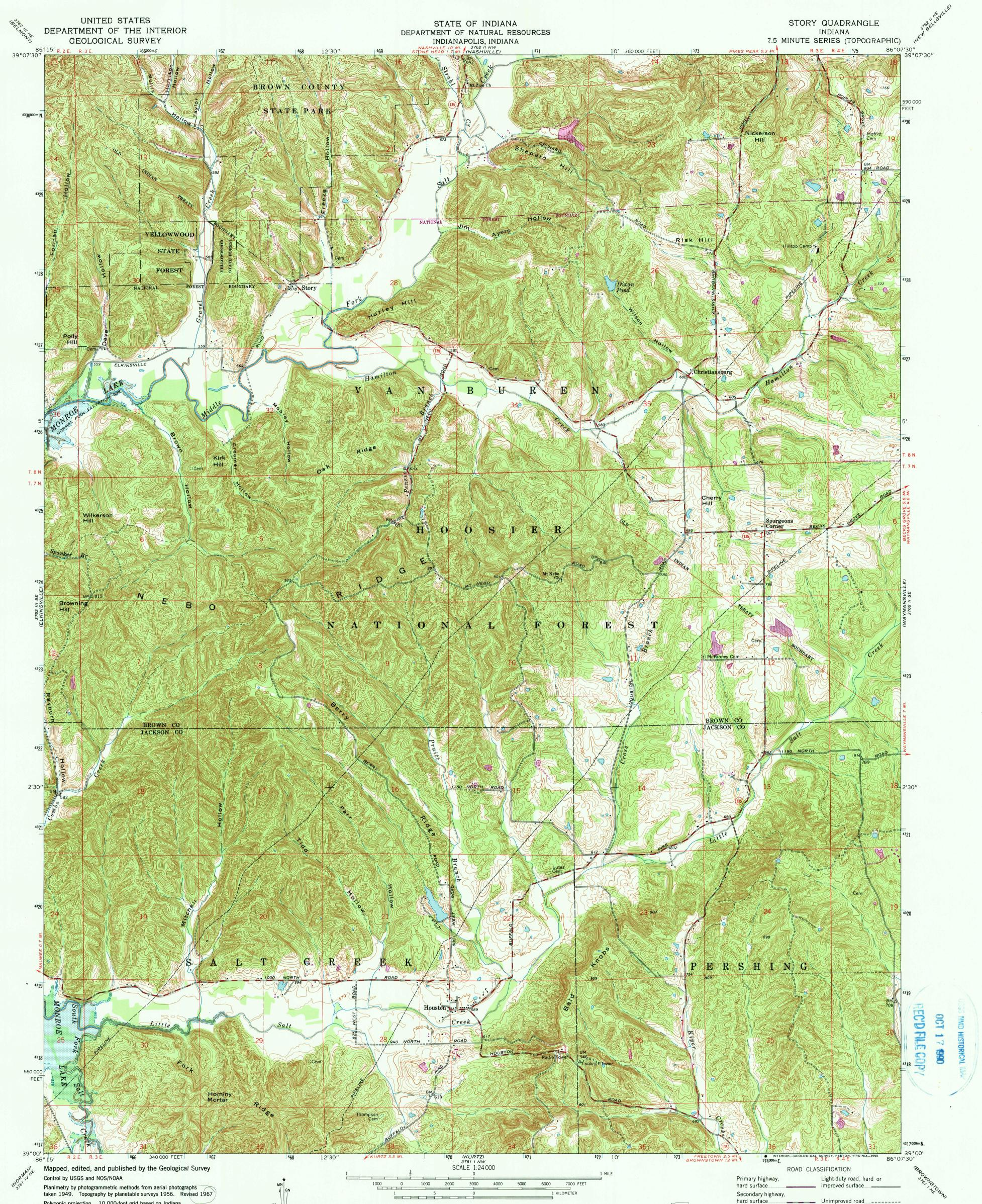
Polyconic projection. 10,000-foot grid based on Indiana coordinate system, east zone. 1000-meter Universal Transverse Mercator grid ticks, zone 16, shown in blue. 1927 North American Datum. To place on the predicted North American Datum 1983 move the projection lines 2 meters south and 1 meter west as shown by dashed corner ticks
