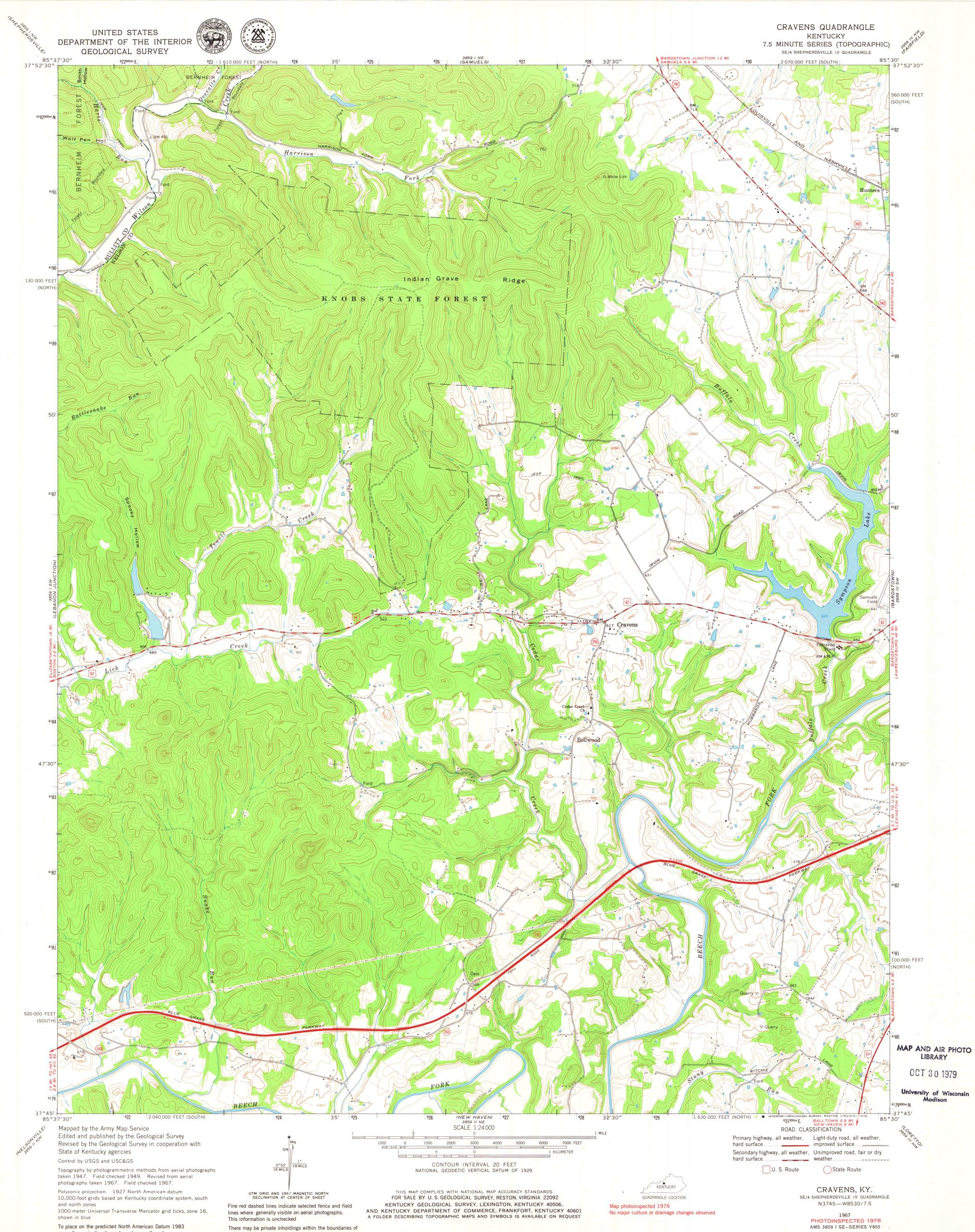
To place on the predicted North American Datum 1983 move the projection lines 4 meters south and 3 meters west as shown by dashed corner ticks
