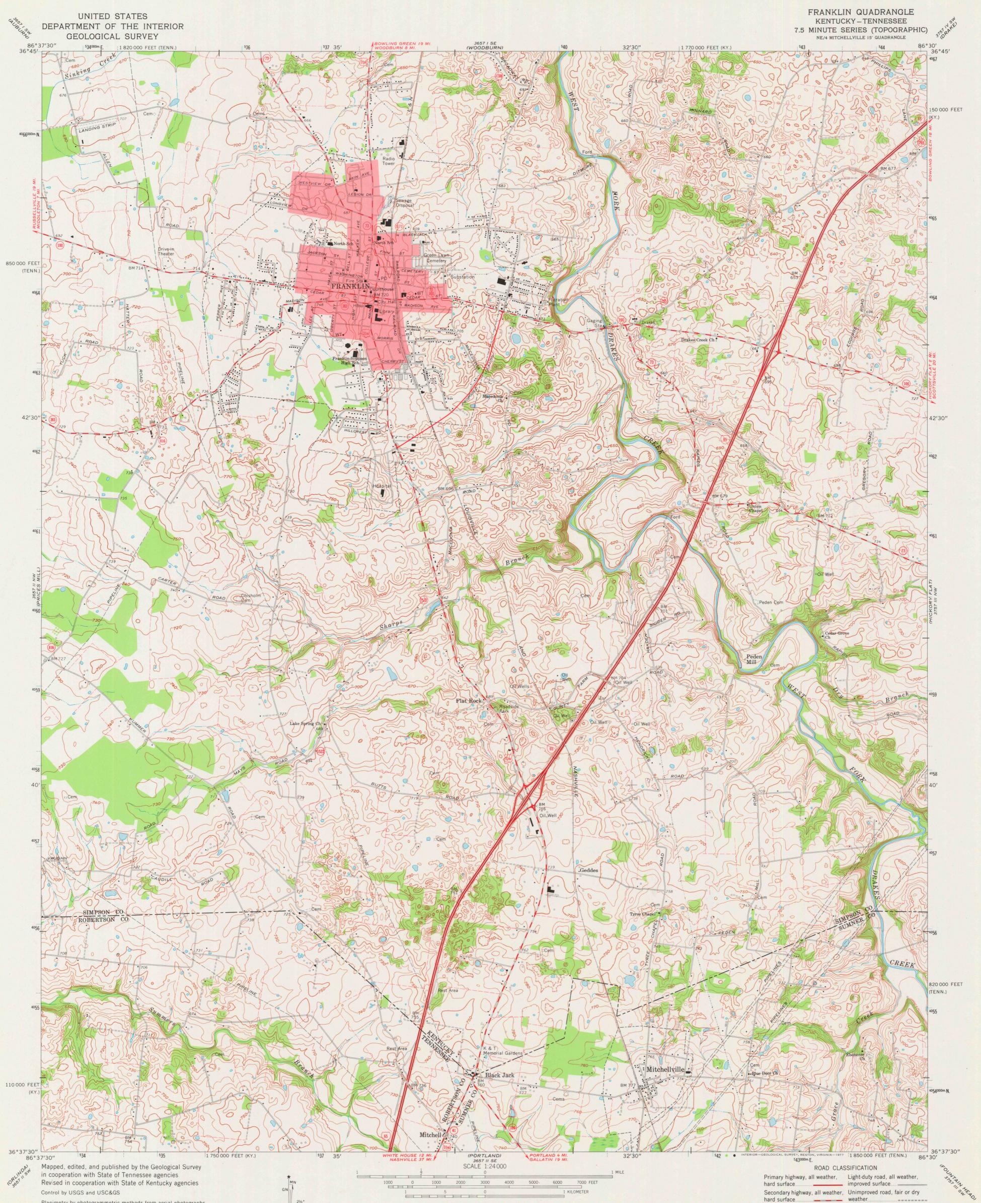
Planimetry by photogrammetric methods from aerial photographs taken 1950. Topography by planetable surveys 1951 Revised from aerial photographs taken 1967. Field checked 1968
