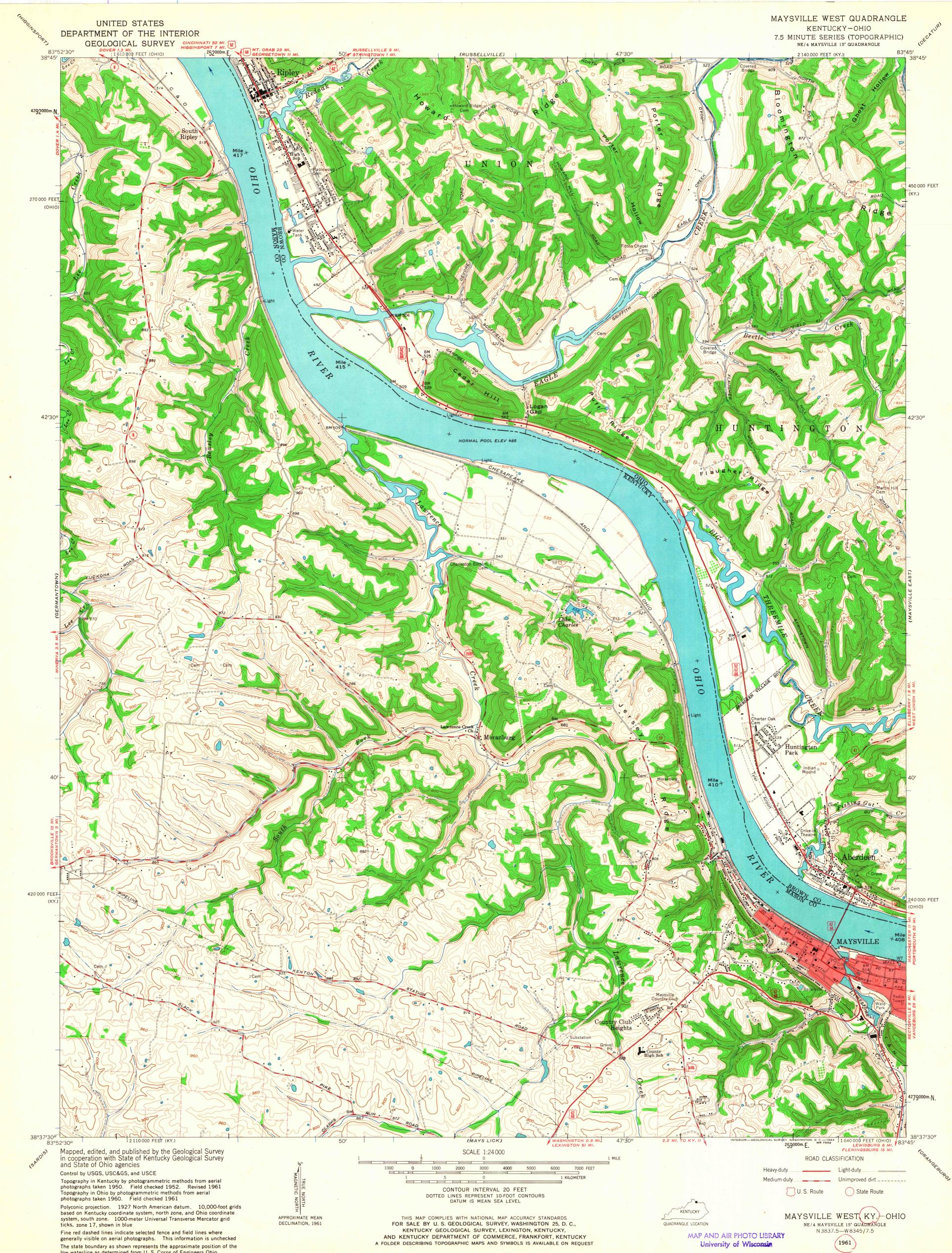
The state boundary as shown represents the approximate position of the low waterline as determined from U. S. Corps of Engineers Ohio River charts, surveyed 1913, and supplementary information Red tint indicates area in which only landmark buildings are shown Ohio area lies within the Virginia Military District
