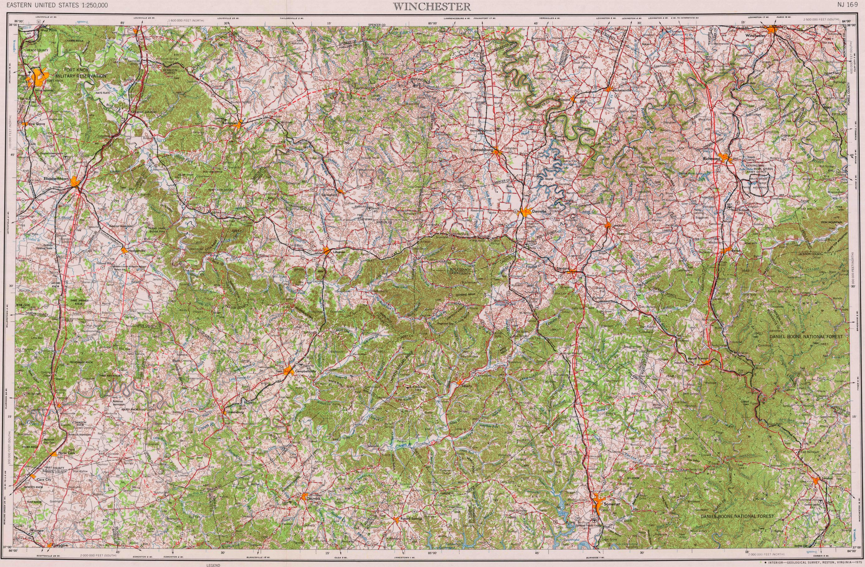
Prepared by the Army Map Service (TVSX), Corps of Engineers, U.S. Army, Washington, D.C. Compiled in 1957 from United States quad-rangles 1:24,000 and 1:25,000, 1947-54. Planimetric detail revised by photo-planimetric methods. Horizontal and vertical control by USGS, USC&GS, USCE, USFS, TVA, and Kentucky Geodetic Survey. Map field checked 1957. Limited revision by U.S. Geological Survey 1967 1967.
