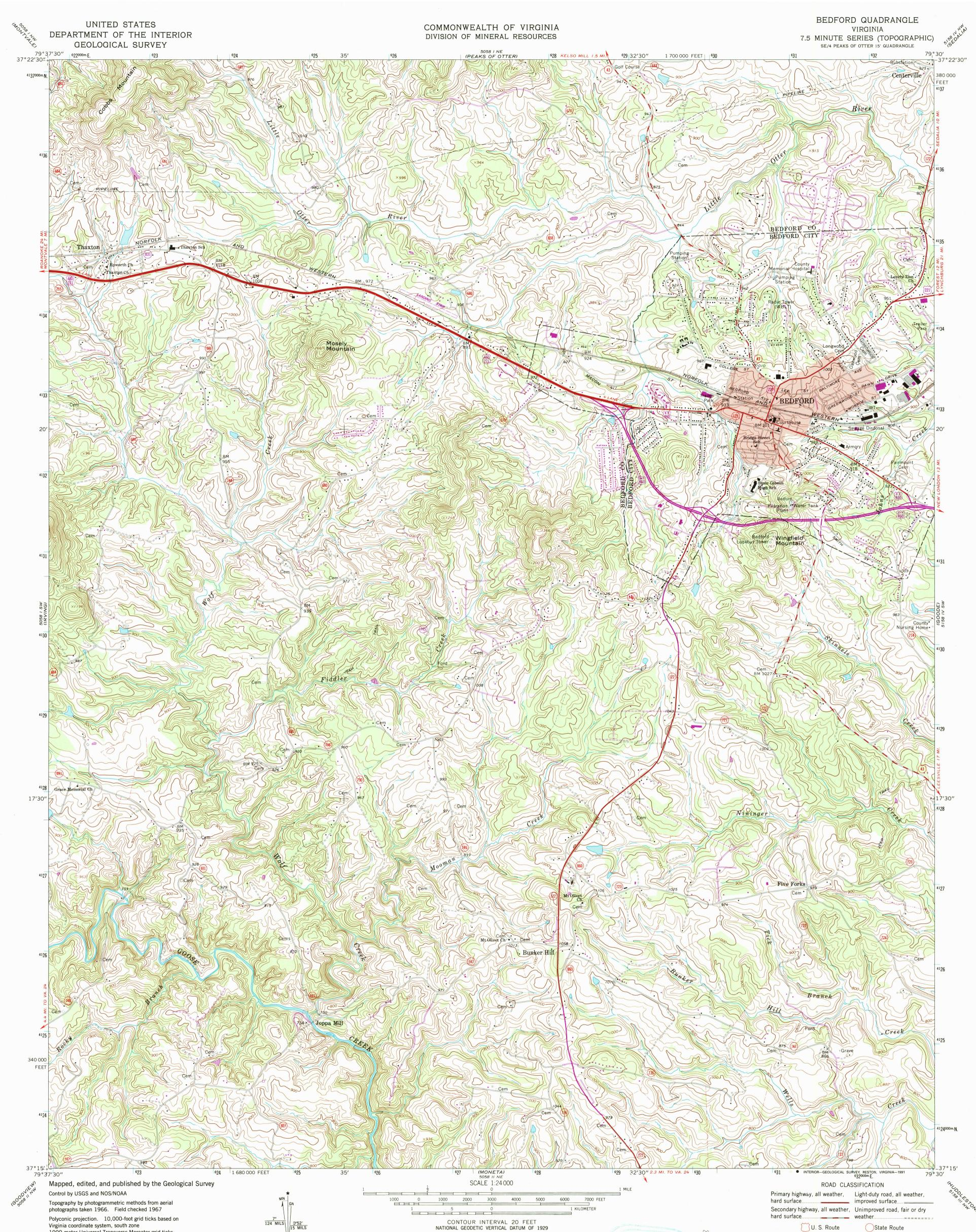
Polyconic projection. 10,000-foot grid ticks based on Virginia coordinate system, south zone 1000-meter Universal Transverse Mercator grid ticks, zone 17, shown in blue 1927 North American Datum To place on the predicted North American Datum 1983 move the projection lines 10 meters south and 21 meters west as shown by dashed corner ticks
