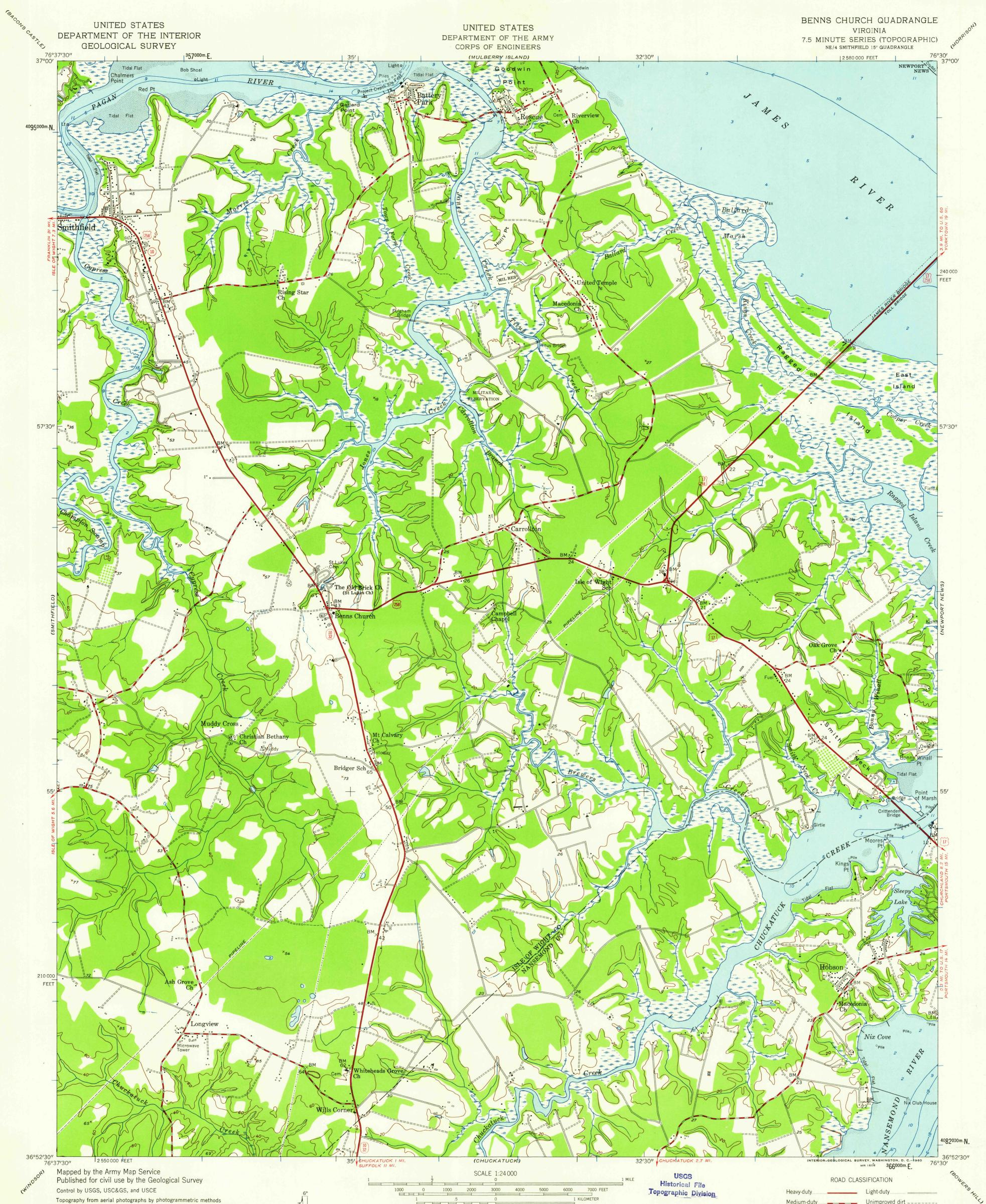
Topography from aerial photographs by photogrammetric methods and by planetable surveys 1943-1944. Aerial photographs taken 1942 Culture and drainage revised from aerial photographs taken 1955-1956 Field check 1957
