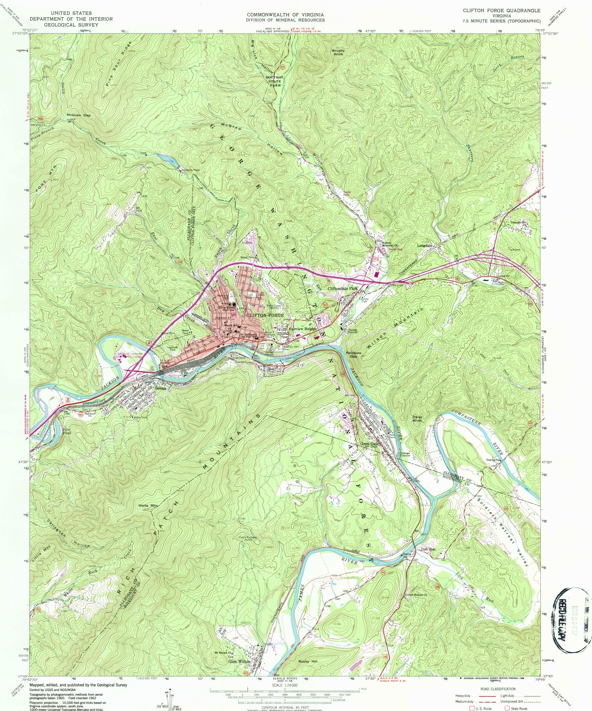
Virginia coordinate system, south zone 1000-meter Universal Transverse Mercator grid ticks, zone 17, shown in blue 1927 North American Datum To place on the predicted North American Datum 1983 move the projection lines 9 meters south and 20 meters west as shown by dashed corner ticks
